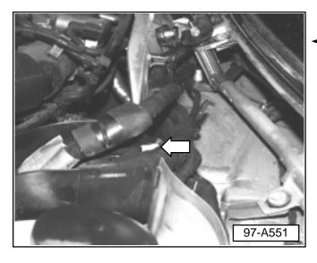
Continue overlay harness routing into left hand harness channel (second assembly mark at plenum as shown (arrow).
