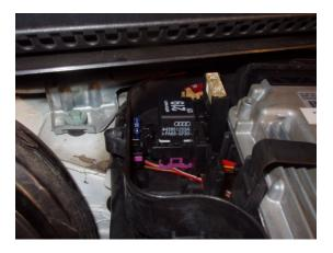
The large 80A fuse is the glow plug fuse (S125).
