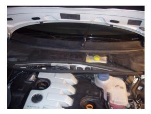
3) Remove plenum cover. Note: some cars have an electrical connector dummied off but attached to the bottom of the cover at the edge of the battery access cover near the positive post.
