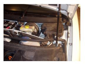
4) Pushing from underneath, remove the screw access plug
