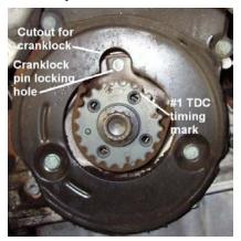
Rotate the engine **clockwise** until the timing mark on the crank pulley is near the alignment pin locking location. This picture was taken before the cover was removed and the engine needed to be turned nearly a full rotation.
