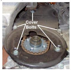
Note: These covers can be removed (and later installed) without removal of the engine bracket, if need be.
