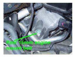
With the engine securely supported, and slightly lifted to ensure the engine is not hanging by the engine mount, remove the 18mm head bolts attaching the body mount to the engine bracket. This sequence is used to lessen the possibility that the removal of the 18mm head bolts will pull out threads from the aluminum engine bracket.
