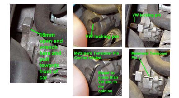
Use a 16mm open end wrench/spanner, or adjustable wrench, on the tensioner tab. Pull towards the front of the car. **Caution:** This is a strong spring mechanism. Insert the locking pin through the holes and remove the wrench. Then slip off the serpentine belt from the tensioner.
