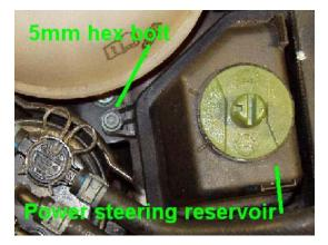
Now you can maneuver the lower coolant bottle hose under the power steering reservoir and move the bottle forward. This will give better access to the upper intake hose clamp.
