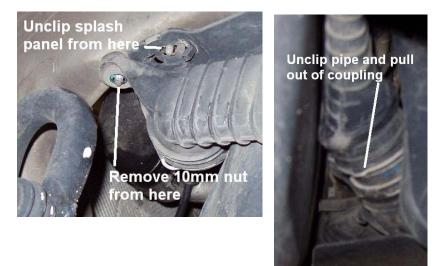
Remove the side splash panel by inserting an appropriate pry tool between the panel and car body at the rear clip (missing from this car) and pry it off of the stud. Then work towards the front of the car and unclip the panel from above the front intake pipe connection. Maneuver the panel out from under the car. Now lower the engine to a point where the entire lower pulley is exposed as pictured below.
