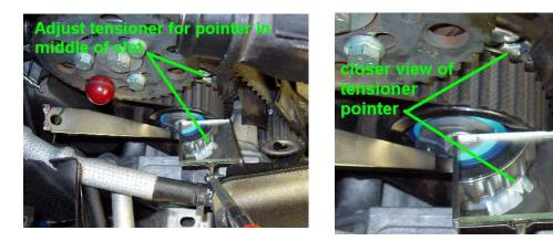
(Note: the tensioner pin holes will be closer to "top" than pictured here. This was "staged".)
