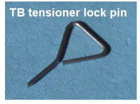
timing belt tensioner pin tool (Metalnerd brand shown)
