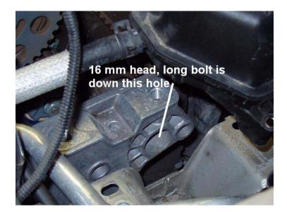
Now remove the long 16mm head bolt from the engine bracket.
