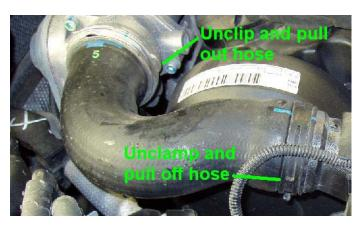
Optionally, the more nimble person can unclip the rigid pipe from behind and below the right headlight, thus removing the entire rigid pipe and hose the entire distance from behind the headlight to the EGR valve.
