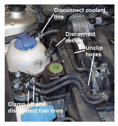
Slide the fuel line hose clamps along the hoses and clamp off the hoses, then remove from the filter with a disposable towel at the ready to catch the small amount of fuel that will leak out. The fuel lines are not pressurized.
