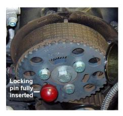
Once the cam is locked, return the crank and turn it until the crank lock inserts into the locking hole. It should not take much, if any. The crank lock slides onto the teeth of the pulley. Do not just lay it on top of the pulley. With everything right, the alignment marks mate up. The knob is removable from the T10050.
