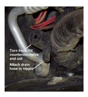
Attach a piece of tubing to the nipple, route to a container, then open the drain by turning <sup>1</sup>/<sub>4</sub> turn counterclockwise and pull out. Open the expansion bottle cap, or remove the cap from the nipple to get it to drain. Tighten the cap, cap off the nipple and blow compressed air into the previously disconnected coolant tube to get more coolant out. Then close the draincock by pushing in and turning <sup>1</sup>/<sub>4</sub> turn clockwise. Remove tubing from draincock nipple.
