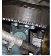
You might get the hole nearly right by turning the crank and then "fine tune" by using a 18mm socket on the cam bolt to vary the cam back and forth until the pin goes into the hole.
