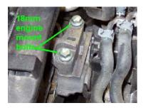
Tighten the 18mm bolts to 74 ft-lbs (100 Nm).
