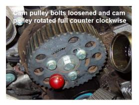
Now install the new timing belt. Loop under the crank pulley first. Then route past the tensioner, and around the cam pulley making sure there is no slack in the belt between the crank and cam. Make sure the belt routes between the tensioner and the engine mount (if the mount is not removed from the car).
