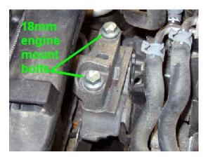
Once these bolts are removed, the 16mm bolts can be completely removed and the engine body mount can be removed from the engine compartment.
