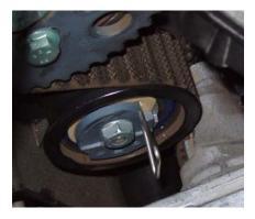
Then turn the tensioner clockwise until it stops and snug up the tensioner nut.
