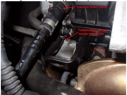
Loosen the clamps on the hoses connected to the EGR cooler and disconnect the hoses. Loosen the clamp holding the coolant hose to the housing above the sensor and disconnect the coolant hose.
