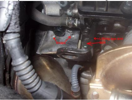
Disconnect the electrical connector from the sensor.
