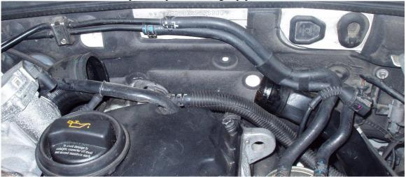
Place the elbow hose retaining clip in the service position as shown. Remove the elbow hose from the throttle.
