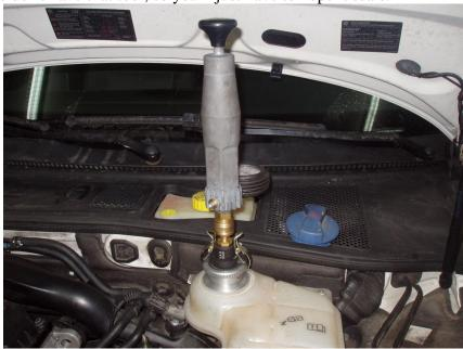
Filling the cooling system is a matter of pouring coolant in, and letting air out. Start by making sure the small hose that connects to the top of the expansion bottle does not have coolant in it. Pull back the heater core hose to allow air out through the bleed hole. Slowly fill the system with coolant until the expansion bottle is filled to the seam.
