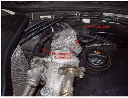
You will want to unbolt the rigid intake pipe near the coolant expansion bottle. This will allow you to more easily remove it from the elbow hose.
