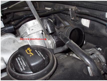
Remove the throttle. There are three bolts attaching the throttle. Use a 8mm triple-square (XZN) bit to remove them. I highly recommend the Metalnerd bit MNXZ8S for this since it is just the right length.
