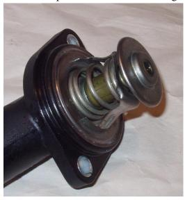
Position the thermostat in the engine block hole, align the bolt holes and press the adapter in until it is flush with the block.
