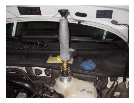
Filling the cooling system is a matter of pouring coolant in, and letting air out. Start by making sure the small hose that connects to the top of the expansion bottle does not have coolant in it. Pull back the heater core hose to allow air out through the bleed hole. Slowly fill the system with coolant until the expansion bottle is filled to the seam.
