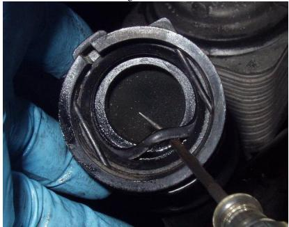
Install a new o-ring in the hose and put the clip back in the installed position.
