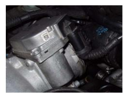
• Disconnect the electrical connector from the EGR valve.
