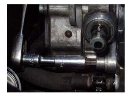
• Finally remove the remaining, easiest to get to, 6mm bolt that attaches the pump to the cylinder head.
