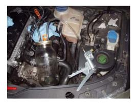
• Using hose clamp pliers, release the feed line from the tandem pump.
