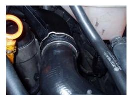
• Use the 10mm socket to unbolt the rigid pipe (in the area of the engine cover holding post).
