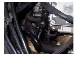
• Now disconnect the fuel lines from the center nipple of the filter, and the return line from the tandem pump at the T on the filter. Have a rag under them to catch any fuel. I prefer to clamp the feed line into the filter to limit drain back to the tank.
