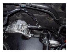
• Disconnect the electrical connector at the large round injector connector at the back of the engine. There should be a small red locking tab that needs to be picked out a short distance before you can turn the connector. It may have been lost if picked out too far before.
