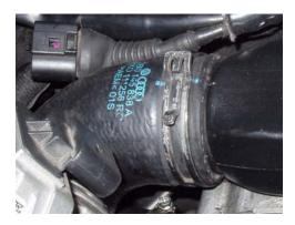
• Disconnect the electrical connector from the intake flap motor.
