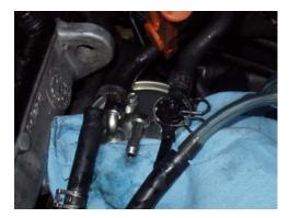
• Using a hand vacuum (or other vacuum source), with an intermediate container, suck the fuel from the disconnected return line. This should suck out most of the fuel from the fuel lines and tandem pump.
