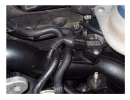
• Disconnect the large flex tubing from the rigid tubing near the oil dipstick.
