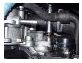
Next remove the 6mm bolt below the large vacuum line nipple.
