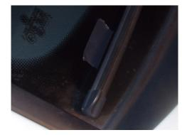
Starting at the edge of the cowl, pry it loose and work across the windshield to near the wiper on the far side. There is a clip in the center that needs to be pulled off. This will allow the cowl to move out of the way enough to remove the battery. If you prefer, repeat the procedure for the wiper removal to remove the other wiper, and completely remove the cowl.
