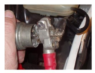
If the brand of battery you install has posts that don't allow the clamps to tighten and stay snug, you can use a battery post shim product such as that pictured here. As of this writing, this product was available at Advance Auto Parts (local stores and internet), and other fine auto parts stores in North America.
