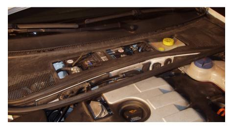
Use a 10mm socket or small wrench to remove loosen the cable clamps and remove the cables from the battery posts. Position them out of the way. Also, pull the battery vent (seen near the positive post) from the battery. Do not pull the vent tube out of the car.
