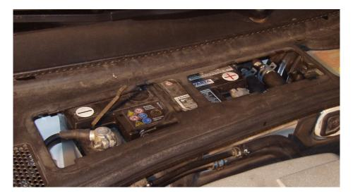
On the right side of the compartment (as pictured above), there may be a battery saver plugged connector clipped to the plenum cover. Gently lift the tab on the clip, then slide the plugged connector towards the battery to release it from the cover.
