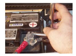
Locate the battery clamp at the base of the battery. Using a 13mm socket, extension and ratchet, remove the bolt and clamp.
