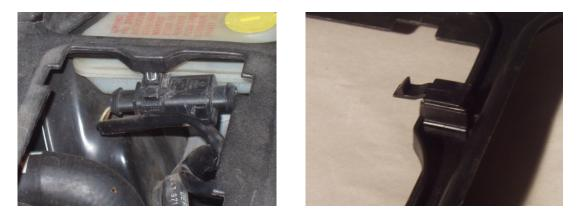
Pull the gasket along the plenum cover loose, and then lift off the plenum cover.
