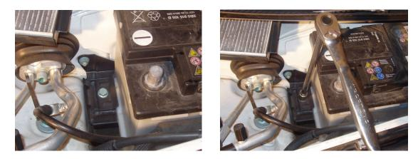
Pry loose the wiper cap, remove the exposed 13mm nut (use the socket and wrench used for the clamp removal), apply a small amount of penetrating oil, let soak a few minutes. While waiting for the soaking, mark the position of the wiper with a small bit of tape. Work the wiper arm straight up and off the tapered drive.
