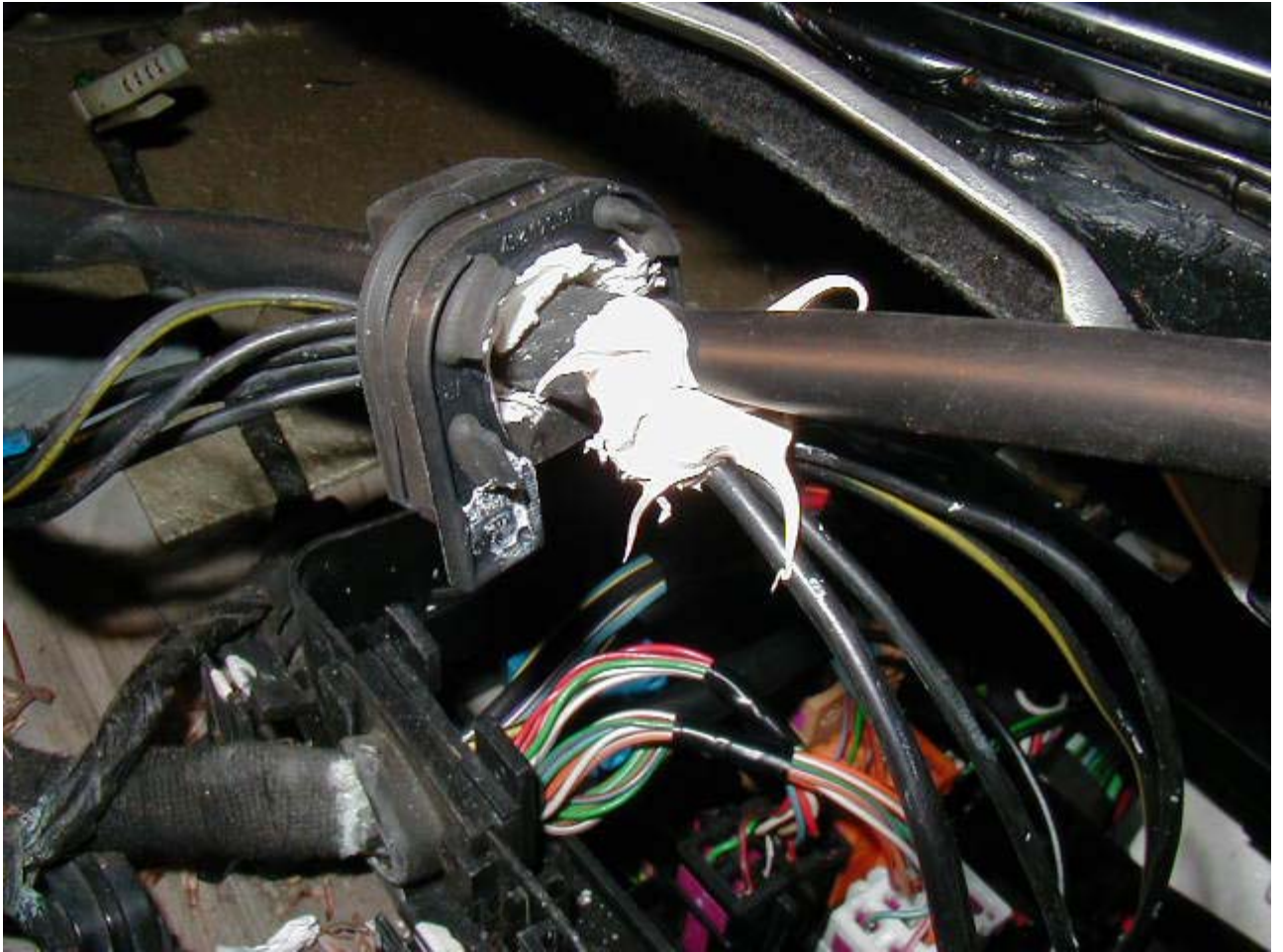
Sealing Wiring through Grommet
