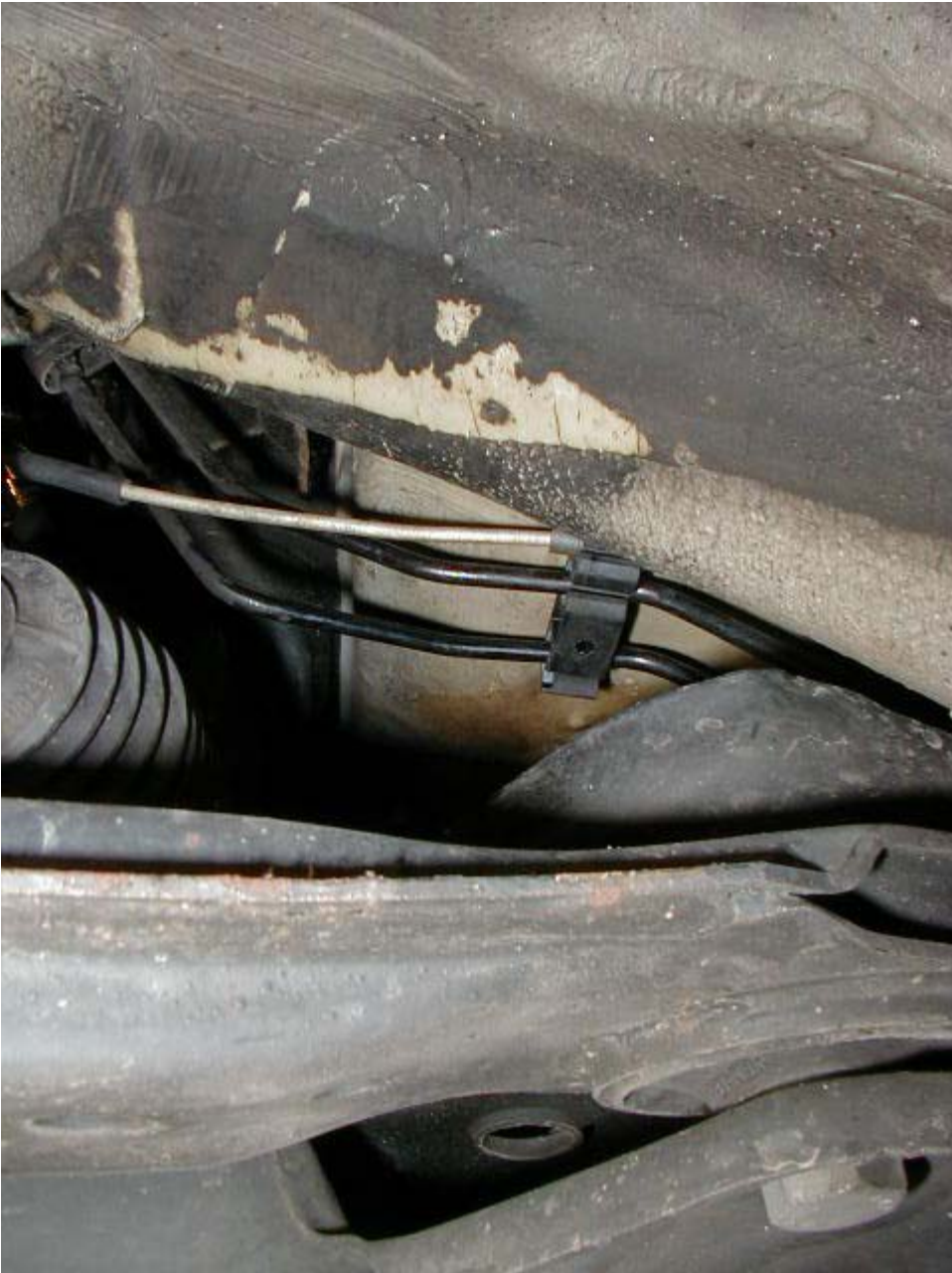
Fuel line with Brake Lines
