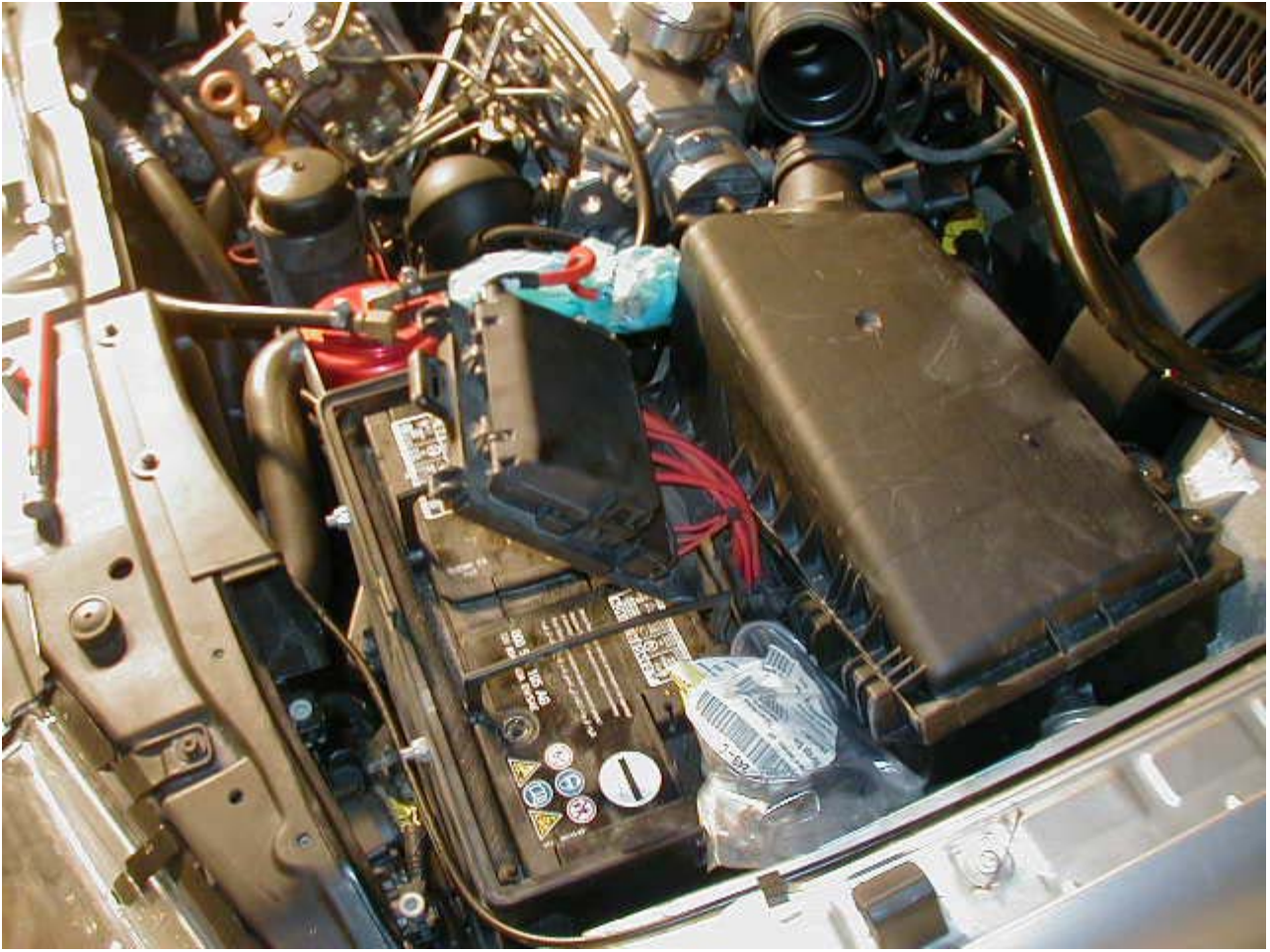
Fuse Holder and Wiring Chase
