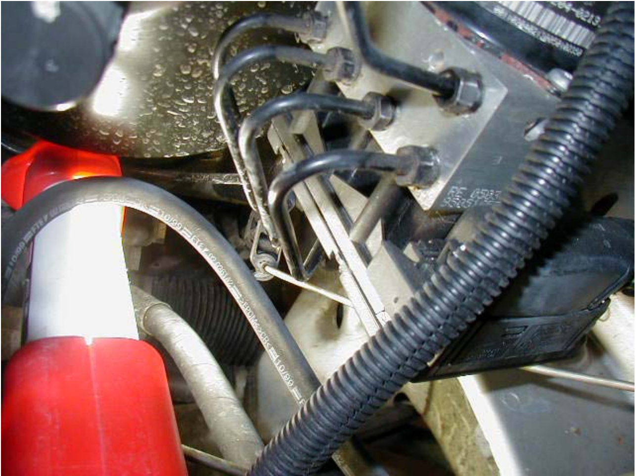
Fuel line under ABS pump
