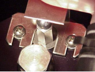
I threaded a 10-32 machine screw in the head of the test plug. I filed off half of the slotted head of the screw so it cannot rotate with the "T" bracket in place. Note that the test plug is rated for 250°F but only 10 PSI pressure. The bracket insures that it won't pop out under fuel pump pressure.
