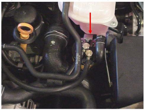
The output line connected to the OEM filter is removed and connected to the output banjo fitting on the CAT filter. This line does not need to be cut or lengthened. An additional 5/16" fuel discharge line is run from the output of the OEM filter to the input of the CAT filter. The thermostat "T" fitting is plugged (not used) on the CAT. Heated fuel in the OEM is fed directly to the CAT filter making this connection unnecessary in this 2 filter arrangement.
