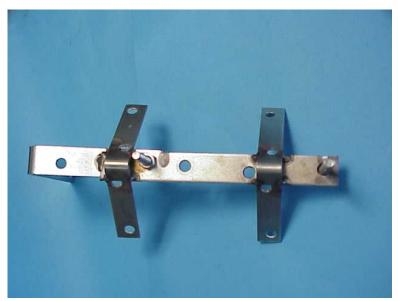
lower mounting bolt hole in the 6" mending brace. The hole is a ¼" thru hole for a 40 mm long 6 X 1.0 mm bolt. The bolt must be metric because it threads directly into a pre-existing threaded bracket in the Passat. This bolt is not welded to the bracket.
