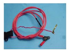
To do this fuel priming the easy way, make a 12 gauge jumper wire that is made from parts obtained from Radio Shack. On one end of the wire connect a small battery clip. An inline fuse holder for a standard size plug-in fuse is soldered on the opposite end of the long wire. A brass tab in this case is soldered to the fuse holder wire so that it can be plugged into the fuse block on the Passat.
