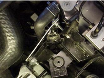
brace. A 5/16" bolt ¾" long is welded to the brace. Note the very shallow bend made in the end of the brace. This end is placed over the upper bolt of the bracket during installation. A hole to receive the bolt is already stamped in the vehicle bracket. The brace is shown installed in the photo above right. I used split washers behind each nut on the bracket to prevent the bracket from coming loose.
