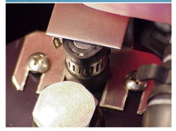
arms on the bracket. I used 1 ½" lengths of Santoprene elastomer tubing (1/2" OD X 3/8" ID) available from McMaster-Carr (catalog # 51225K35). This stuff has high surface friction and a high temperature rating. Just stretch and slide the tubing on the arms of the bracket. I put heat shrink tubing on the bottom leg of the bracket.
