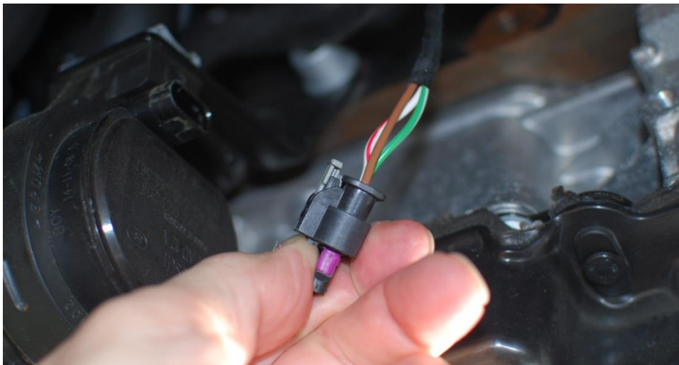
Wire to one of the coolant pumps is in the way. The gray clip pulls back with a slight click, then the connector pulls straight out of the pump.
