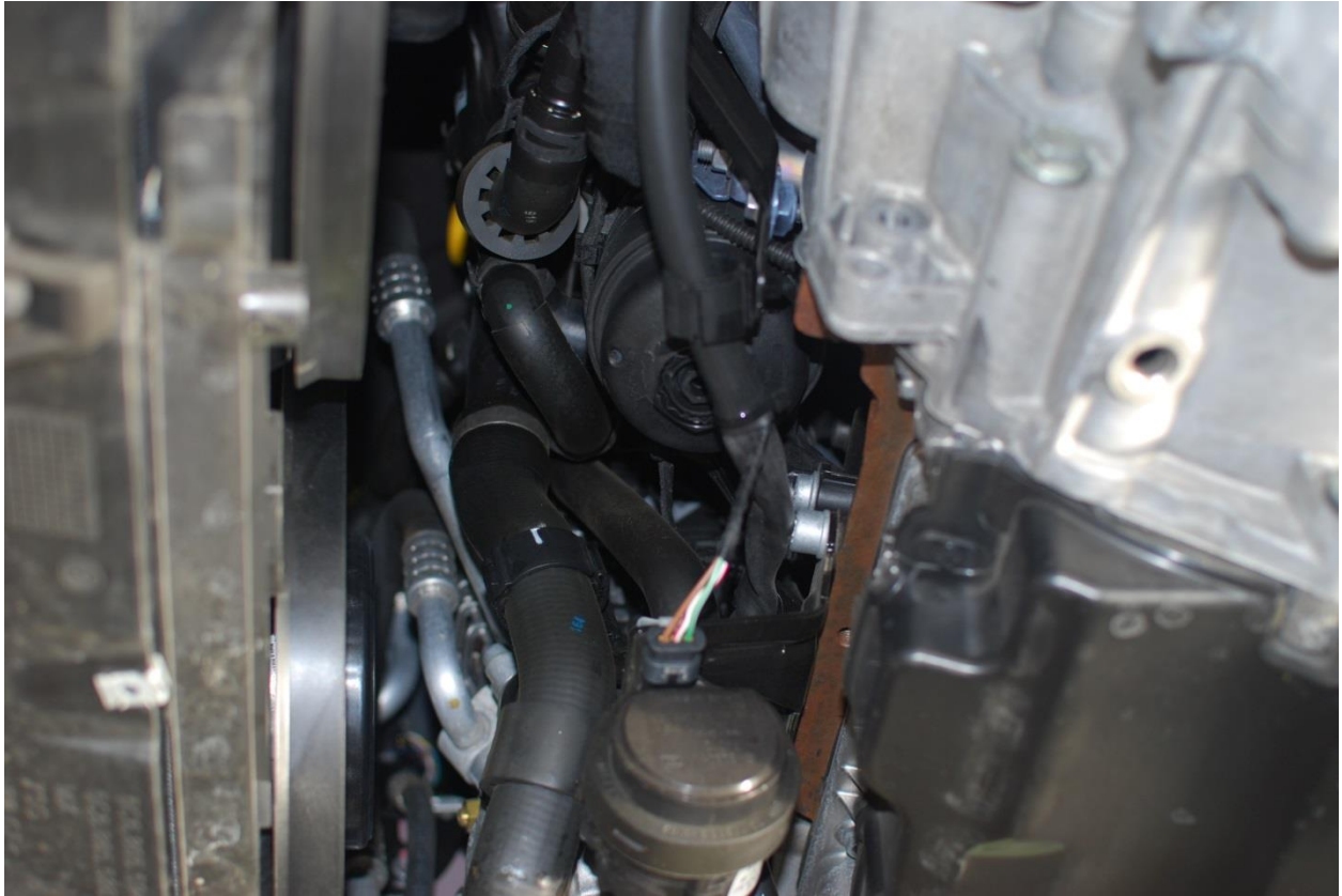
There is the oil filter hiding in front.
