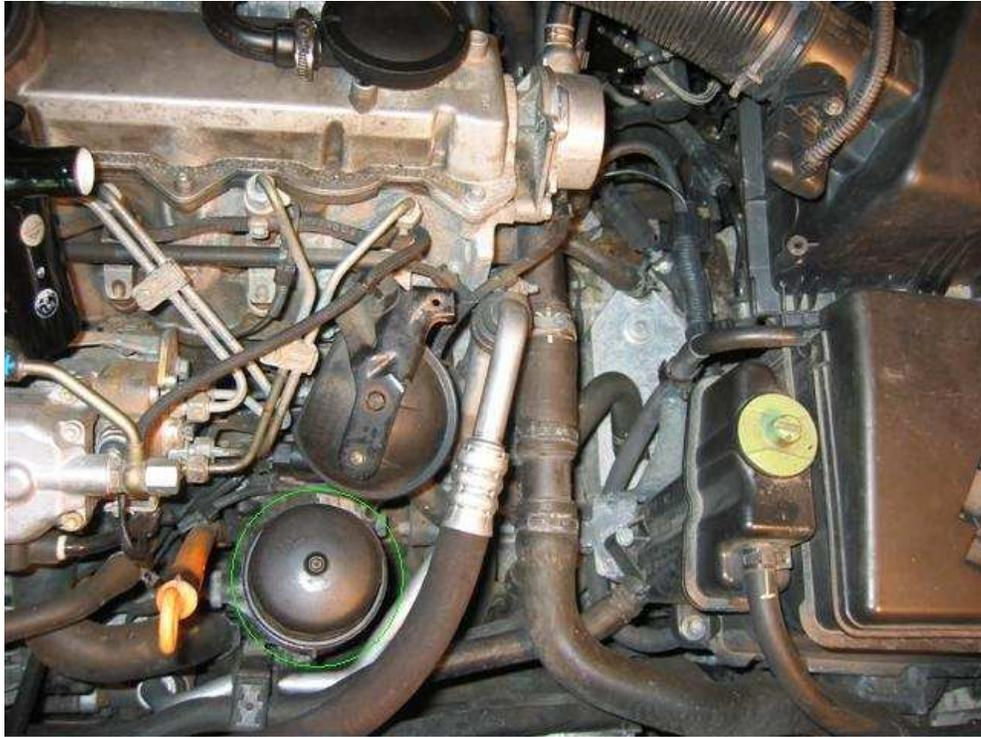
The oil filter housing is the one with the green circle. Use the flute oil wrench or strap to remove it. I suggest having paper towels and/or paper bag next to it. Once you have loosened the cap completely, pick it up and allow the oil to drip from it before you move it.
