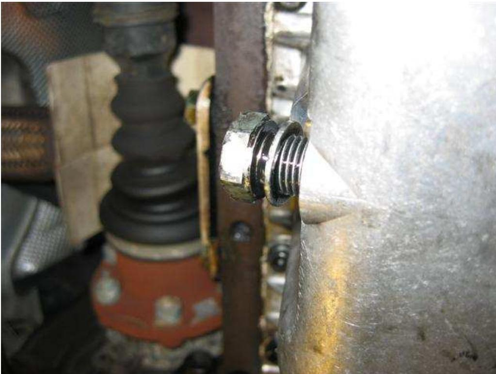
When the oil is done dripping, wipe up the area and clean the plug. Carefully and gently, hand screw the plug in the pan. Don't force it. You don't want to cross thread it. Once it is on correctly, fully hand tight it. With the torque wrench, tighten it to 22 ft/lbs (30 Nm.)
