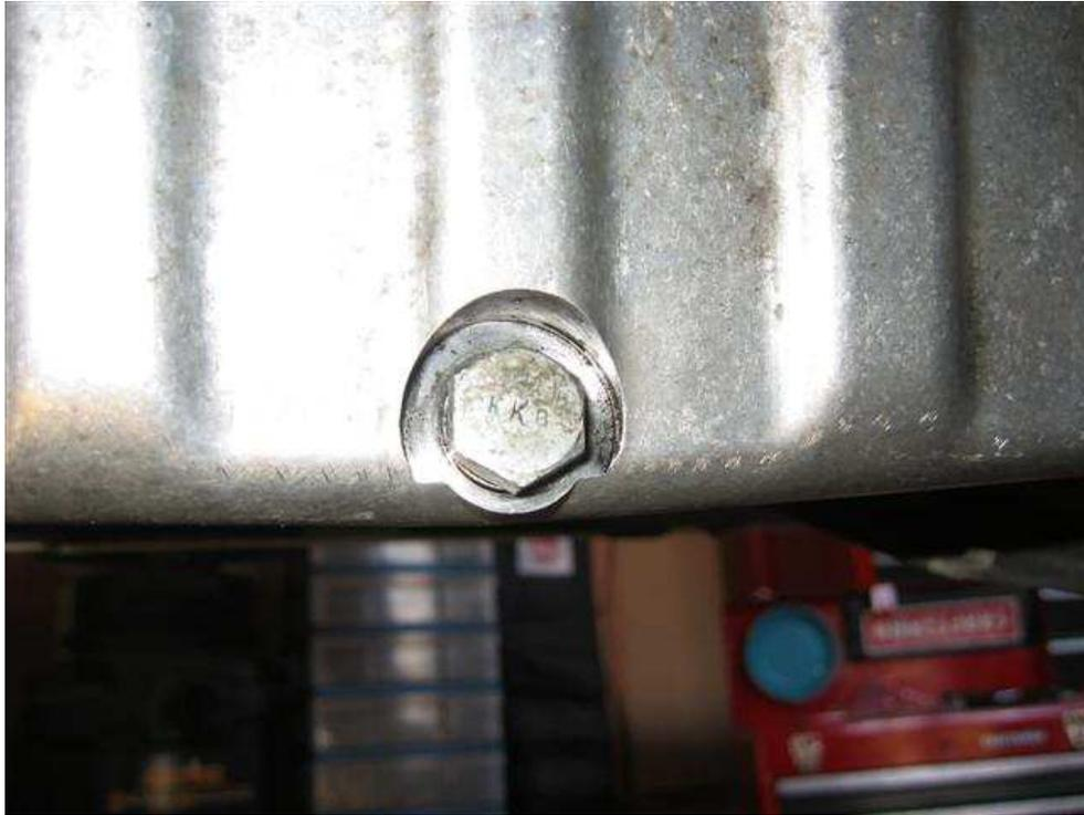
Get the 19mm socket or wrench and loosen the oil drain plug. Just loosen it so that you can remove it by hand after you position the oil drain pan under. I strongly suggest wearing a latex glove. With the pan under, remove the drain plug. The oil will come out. Let it drain. Let's work on the filter. (Notice the drain plug on the left of the pan below my white dirty fingers.)
