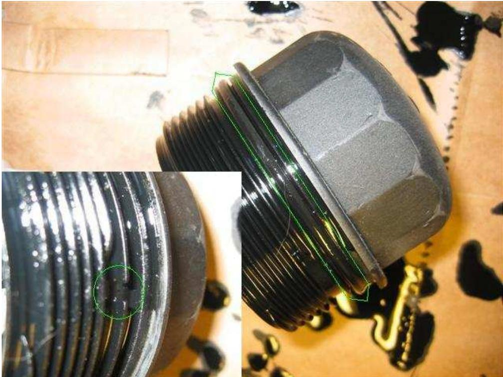
Remove the large O ring with the needle nose pliers. There is a notch on the cap that will assist you to get the ring removed easy with the pliers.
