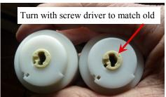
Make sure the hole in the end of the new switch is keyed in the same orientation as the old one (turn with blade screw driver if needed), then slide the new one into the housing . It should go in easily and be flush with the housing.
