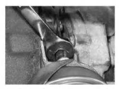
$\bullet$  Tighten lock nut to 6 Nm (53 in. lbs.) while using an 11 mm wrench to counter-hold the adjustment arm . This prevents the adjusting rod from twisting during the tightening of the nut.
