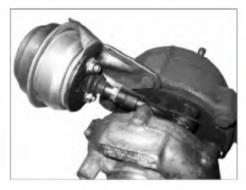
· Install new actuator tighten nuts to 6 N.m (53 in. lbs), install new snapring / cir-clip.
