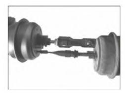
· Adjust the new actuator to same length as original, as shown above, to obtain initial adjustment.
