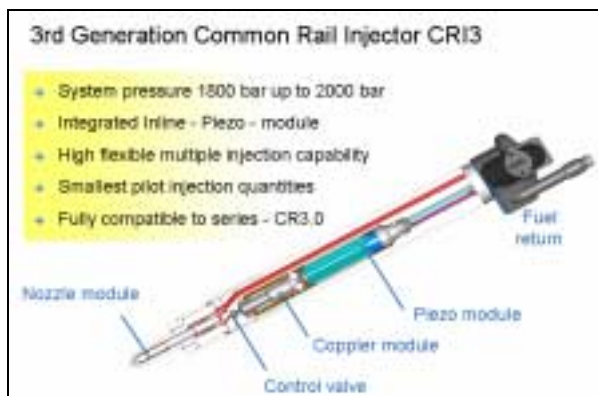
Figure 6: 3 rd Gen. Common Rail Injector CRI3
