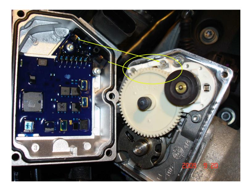
=> Make both gaps smaller to improve the electrical contacts. I used a small nail and lift both tabs up on each of the 2 "female sockets"
