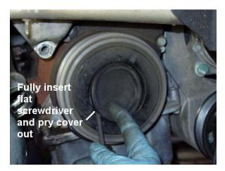
To remove the damper you will have to counter hold the crank with a 19mm 12-point socket and breaker bar, while using a 6mm hex bit socket on the bolts. These are fairly snug and may take some effort to remove. If hard to remove use an Irwin Bolt-Grip, or Sears Craftsman Bolt-Out, to remove. If this is the second timing belt replacement, plan on replacing the bolts.
