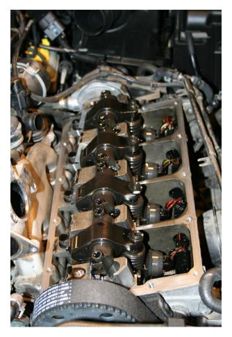
Loosen the M10 triple square bolts on the injector rocker shafts and remove...keep them in order! Loosen them slowly and evenly. They will come out in two pieces, four bolts each. Remove the cam locking pin, and the cam pulley. Use a special gear puller, carefully hammer on the pulley, or use your imagination to get it off. If it doesn't come off easily, don't worry about it. Make sure the belt is off the pulley and start working on the bearing caps.
