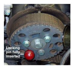
Once the cam is locked, return the crank and turn it until the crank lock inserts into the locking hole. It should not take much, if any. The crank lock slides onto the teeth of the pulley. Do not just lay it on top of the pulley. With everything right, the alignment marks mate up. The knob is removable from the T10050.
