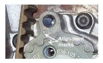
From above, loosen the tensioner bolt (but don't remove) and use the tensioner tool (or 5mm allen wrench) to adjust (loosen) the tensioner counter clockwise until the tension is released from the timing belt. If it's loose enough, slide it off of the crankshaft pulley, and then off of the cam. Again, be careful to work around the belt and not damage it. If your belt is due for a change, now would be the time to do it! Follow MOGolf's timing belt R&R instructions.
