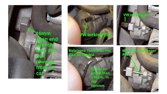
Now remove the three bolts securing the tensioner with a 13mm socket wrench, and remove the tensioner.
