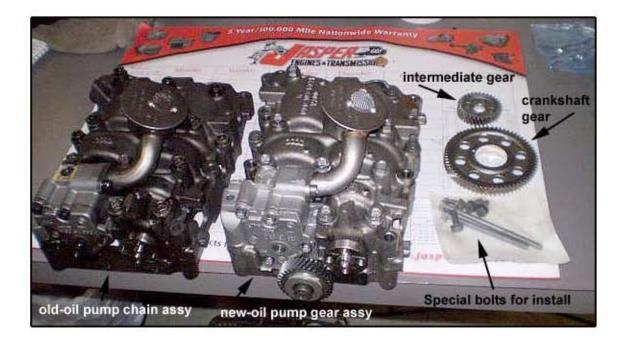
This is a side by side comparison photo of the older oil pump chain and the oil pump gear along with assorted parts for the conversion.
