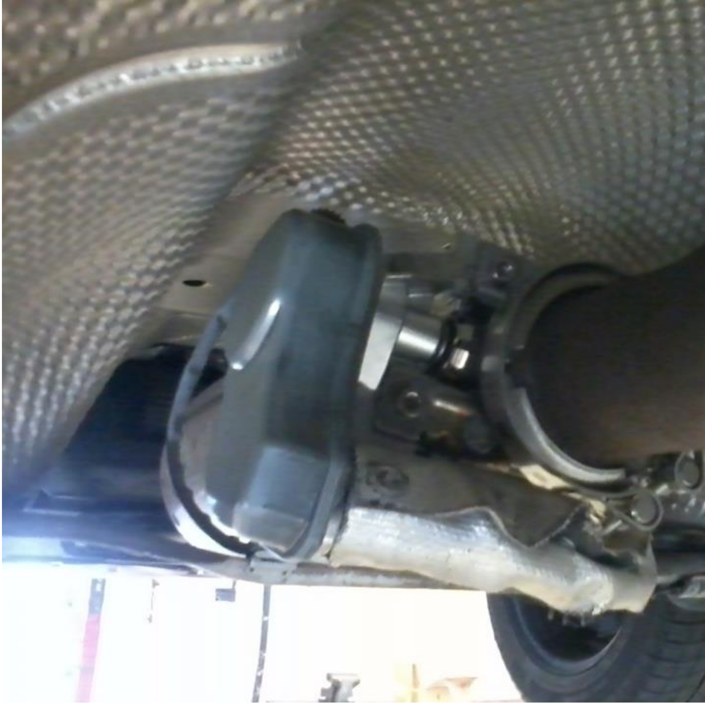
Here is a shot of the flap under the car. note the wiring is protected by wrap which snaps together, and the VW exhaust clamp.
