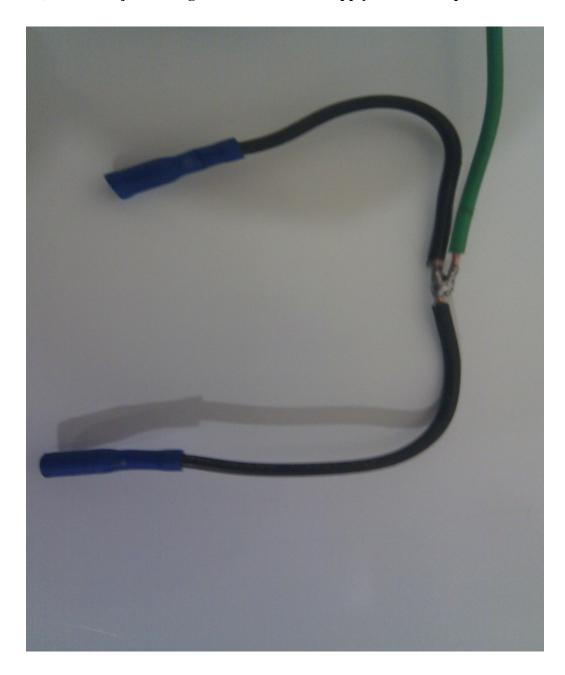
Next, solder the joints for good connection and apply electrical tape on them.
