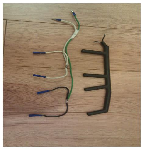
First, cut the wires to approximate size laying next to oem harness.
