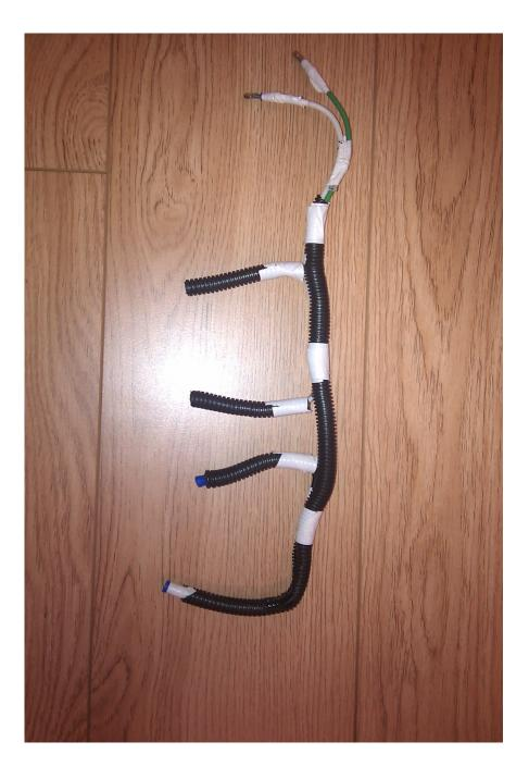
I also connected 2 female connectors on the car side wires. Here is my \$2 glow plug harness installed in my car. It is working perfectly for more then six months now.
