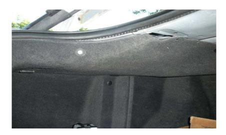
2) As the wire given with the 30 LED strip will typically not reach the stock trunk light, you will need to add wire to each side. Using your 30 LED strip, mock up the position that you permanently want the light installed, and measure how much wire you will need to reach the factory trunk light.
