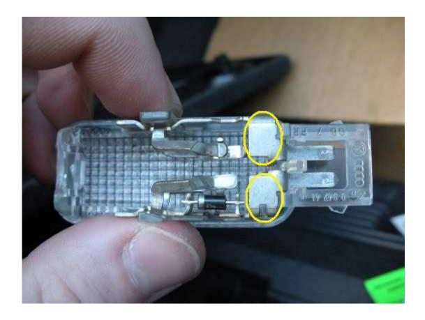
6) Now, route your LED light through the trunk light hole and install the trunk light with a working bulb. If you're using the light strip from superbrightleds.com, it will come with 3m adhesive on the back. Peel the adhesive and install where you prefer. I mounted it under the front lip of the trunk and it is well hidden while looking at it from the outside.
