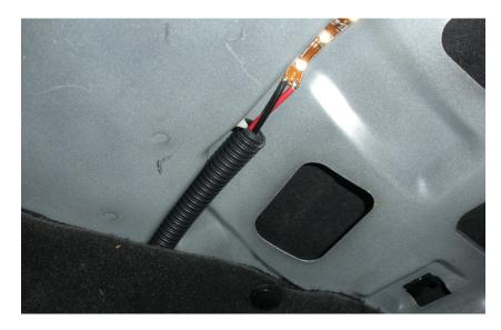
8) Re-connect the electrical connector and make sure the light works as it should and re-install the trunk liner. Now sit back, and enjoy the fruits of your labor! PROST!
