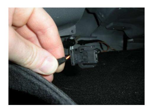
5) Next, using the measured lengths of wire from the mock-up, solder one wire to the B+ terminal and the other to the ground terminal on the back of the light. Then solder / crimp connect the other ends to the corresponding B+/Gnd side on the light. See the diagram and pictures below.
