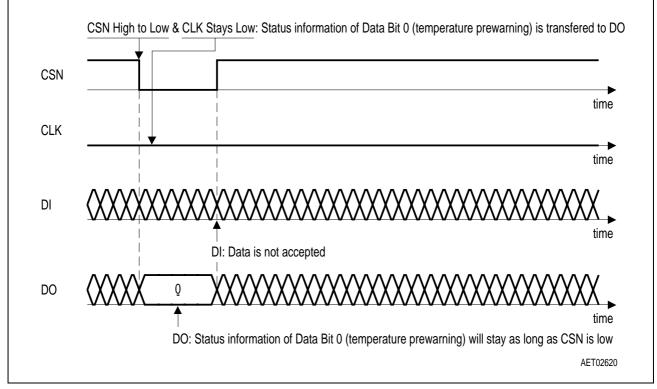
Figure 4 Timing for Temperature Prewarning only
