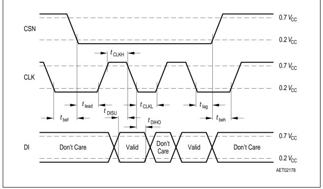
Figure 5 SPI-Input Timing
