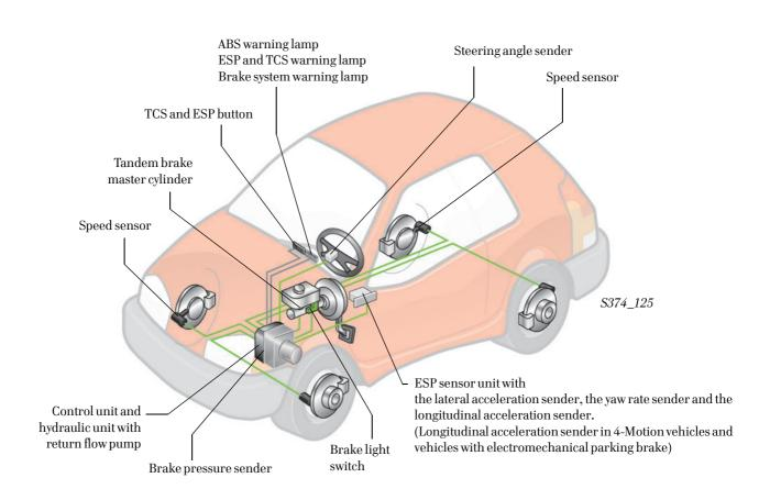
The system's sensors are sub-divided into the senders for registering the driver's command and those for sensing the vehicle behaviour.
