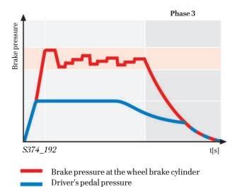
If the driver reduces the pedal pressure or negative deviation from the minimum speed occurs, the trigger conditions for the HBA are no longer given. The ABS/ESP control unit recognises that the emergency situation has been averted and begins to end brake assistance. The brake pressure increased by HBA is gradually reduced until it is again adapted to the driver's pedal pressure.
