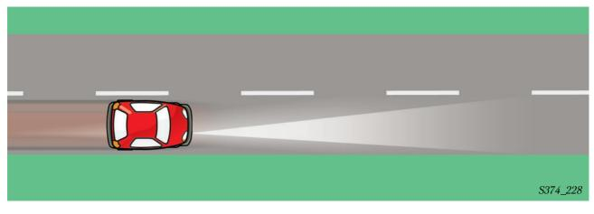
No vehicle is located in the proximity control sender's field of vision.
