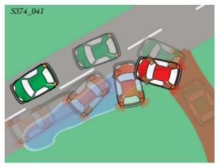
In the event of full braking on the wet road surface, the wheels lock up. The vehicle begins to skid.
