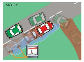
Reducing the brake pressure at the wheels on the wet road surface prevents the wheels from locking up. It remains possible to steer the vehicle.
