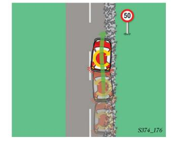
In a vehicle with countersteering support, correspondingly targeted steering forces are applied via the power steering system to support the driver in countersteering. As a result of this, the stopping distance is reduced, there is less deviation from the course and the vehicle's stability is increased.
