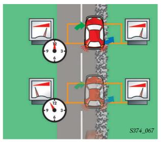
The brake pressure at the wheels on the surface with better grip does not increase so quickly. The dangerous yaw rate is overcome.
