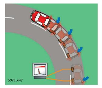
In vehicles with CBC, the brake pressure at the inner wheels is reduced in the event of oversteering. This increases the wheel location forces at the inner wheels and the vehicle's rear end remains stable.
