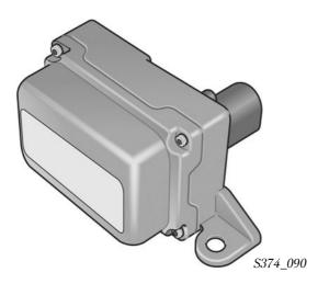
This sensor unit is a combination of the lateral acceleration sender G200, the longitudinal acceleration sender G251 and the yaw rate sender G202. Both acceleration sensors operate according to the capacitive principle and differ only as regards the sensors' spatial orientation to the relevant acceleration direction.
