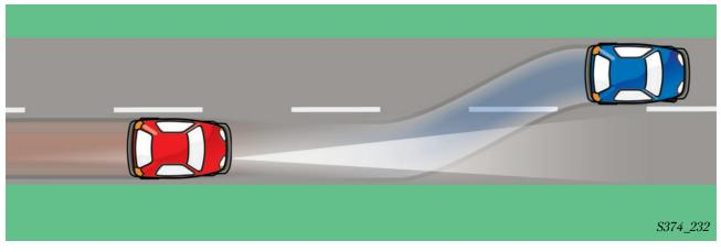
The distance becomes greater than the desired distance, because the preceding vehicle accelerates or clears the way by changing lanes.
