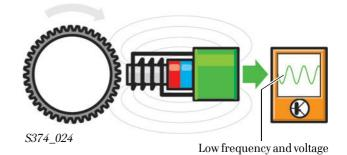
Sensor signal at high speed
