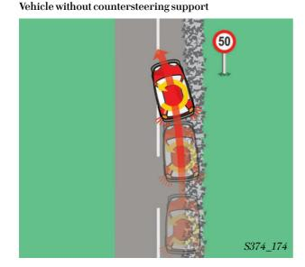
In a vehicle without countersteering support, the time and extent of countersteering support are determined solely by the driver. In the case of inexperienced drivers, this may lead to excessive steering movements, which may result in an unstable driving situation.
