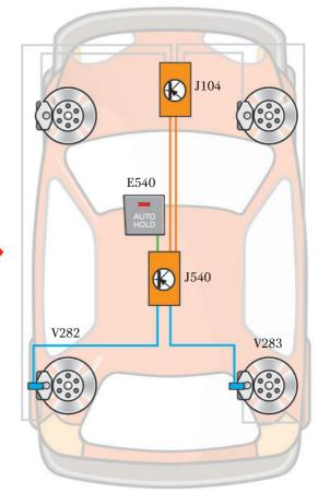
Legend E540 AUTO HOLD button J104 ABS control unit J540 Control unit for electromechanical parking brake V282 Left parking brake motor
