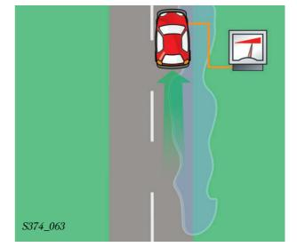
The wheel on the wet road surface is braked and the slip is limited. As a result, the drive power is increased via the differential and transmitted to the wheel which is not spinning. The vehicle with EDL reaches a higher speed in the same time.
