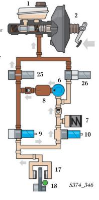
In order to then build up the pressure again gradually, the switch and the outlet valve are closed again and the high-pressure valve is opened. The return flow pump is actuated and begins pumping. The inlet valve opens and closes at brief intervals, and the brake pressure can therefore be increased gradually.
