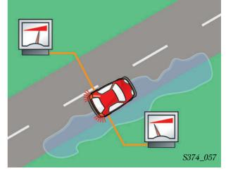
Different brake pressure distribution between the two rear wheels due to different road surface conditions
