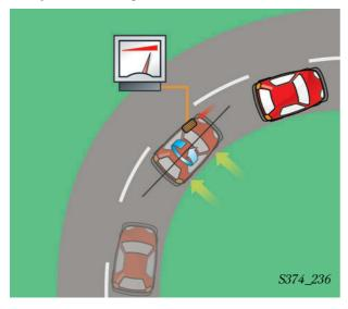
To stabilise the vehicle, the outer front wheel is specifically braked via ROP intervention.
