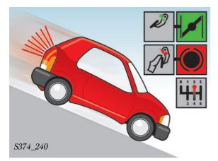
A driver in a vehicle without hill descent assist system must therefore brake manually, shift to a lower gear and release the accelerator in order to maintain a constant vehicle speed.
