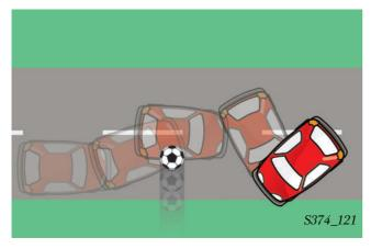
The vehicle without ESP has to evade an obstacle which suddenly emerges. The driver first steers very quickly to the left and immediately afterwards back to the right. The vehicle begins to sway due to the preceding steering movements, and the rear end breaks away. The rotation around the vertical axis can no longer be controlled by the driver. The vehicle begins to skid.
