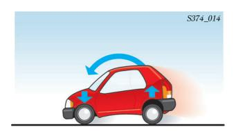
Due to the pitching motion on braking, the axle load at the front axle is increased and the rear axle is relieved.
