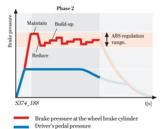
ABS intervention keeps the brake pressure below the lock up threshold. Regulation takes place in three phases: "Maintain pressure", "reduce pressure" and "build up pressure".
