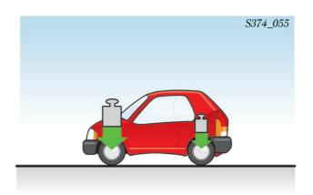
Due to weight distribution in the vehicle, rear axle wheel load is significantly lower than that on the front axle. To achieve controllable vehicle dynamics, brake pressure distribution has been defined such that the front axle brakes should lock up before the rear axle brakes (Directive ECE13; ECE=Economic Commission for Europe), in order to maintain residual vehicle stability in the longitudinal direction.
