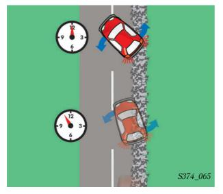
The side of the vehicle on the surface with better grip is braked more extensively than the side of the vehicle on the smooth surface. The yawing moment which occurs in this case causes a yaw rate, which the driver cannot compensate quickly enough via the steering.
