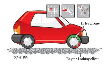
Under unfavourable conditions in the case of vehicles with very high-powered engines, the engine braking effect may lead to the wheels' locking up or to such extensive slip that lateral guidance forces are lost and it becomes impossible to steer the vehicle.
