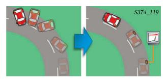
On oversteering, the outer front wheel is braked.
