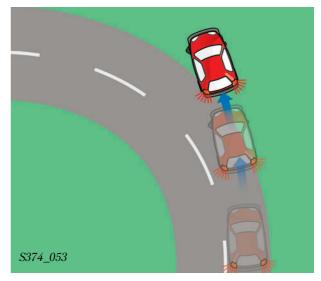
If a vehicle without CBC is braked extensively on cornering, the wheel location forces on the front wheels are reduced. The vehicle pushes over the front axle towards the outer edge of the curve.
