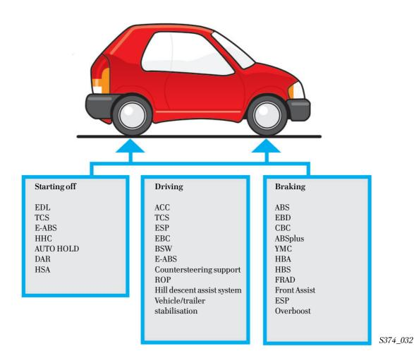
A further and more detailed option for classifying them is to sub-divide the traction control systems into two groups. Firstly, those systems with brake intervention solely via the hydraulic brake system and secondly, those which additionally influence vehicle dynamics via the engine management system or gearbox management system.
