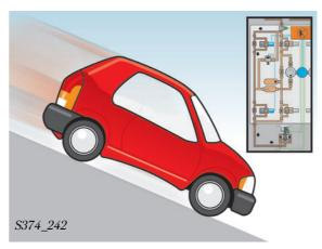
A vehicle with hill descent assist system relieves the driver of this manual intervention and ensures that the desired speed is also maintained whilst descending the hill.
