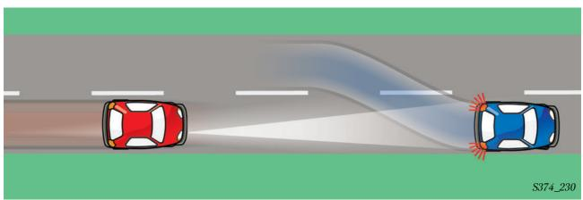
If the distance becomes less than the desired distance, because the preceding vehicle brakes or a slower vehicle moves in front by changing lanes, the vehicle is braked to the pre-selected desired distance. This deceleration may take place via intervention in the engine management system. If deceleration via the engine torque is not sufficient, brake intervention takes place. The systems fitted in the Touareg can brake the vehicle to a standstill if the traffic situation necessitates.
