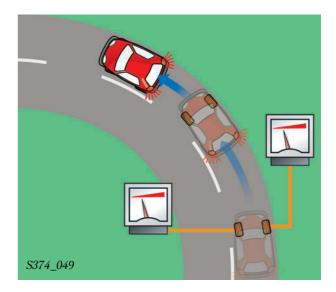
In vehicles with CBC, the brake pressure on the front axle is reduced in the event of understeering. As a result, the wheel location forces are increased and the vehicle remains on course. Oversteering
