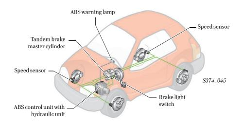
Splitting the brake system into two separate brake circuits increases the vehicle's safety. If one circuit fails, the vehicle can still be brought to a stop via the second brake circuit.
