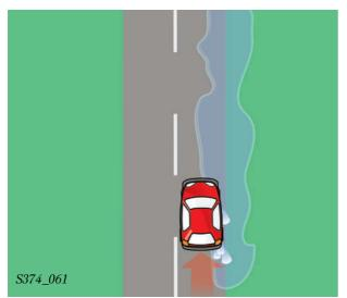
The vehicle can only be accelerated with the drive power transmitted to the spinning wheel, because the differential is able to pass on only the smaller of an axle's two drive torques. The vehicle is only able to accelerate very slowly.
