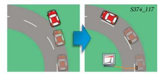
On understeering, ESP prevents departure from the curve by specifically braking the inner rear wheel.
