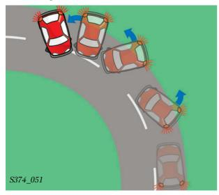
If a vehicle without CBC, which enters a curve at an excessive speed, is steered and braked too severely, the rear end breaks away to the outer edge or the curve.
