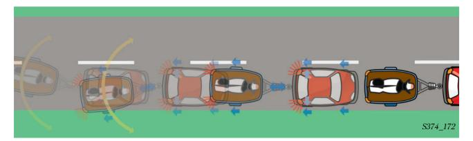
The vehicle/trailer stabilisation system is an extension of the ESP regulation system's software, which overcomes this danger. The vehicle/trailer combination is initially stabilised via brake intervention on alternating sides of the towing vehicle. If this is not sufficient, all four of the towing vehicle's and the trailer's wheels are braked via the trailer's inertia brake for stabilisation purposes.
