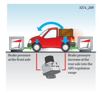
The FRAD function enables a maximum rear axle braking effect.
