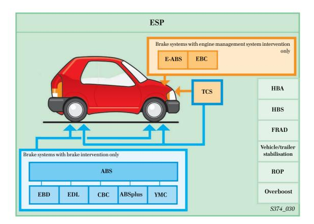
The anti-lock brake system ABS is the source of all traction control systems, and is a brake system with brake intervention only. The software extensions and extensions via additional ABS system components include EBD, EDL, CBC, ABSplus and YMC.
