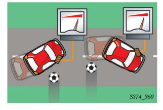
The risk of tipping-over during dynamic swerving manoeuvres on road surfaces with good frictional adhesion is high for almost all vehicles. This manoeuvre is recognised and, although the vehicle is not yet skidding, very high pressure is built up very rapidly at the relevant, outer front wheel.
