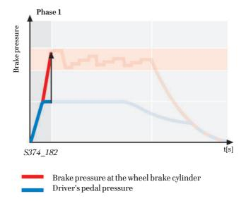
In the hydraulic unit, the switch valve is closed and the high-pressure valve is opened. The return flow pump is actuated and begins pumping. As a result of this, the pressure at the wheel brake is increased to the maximum, over and above the brake pressure triggered by the driver. If the wheels are in danger of locking up, ABS intervenes.
