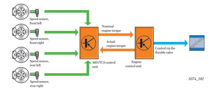
E-ABS is unable to intervene hydraulically in the drive wheel brake cylinders. The system does not have the option or equipment to independently build up brake pressure via a pressurisation system without the involvement of the driver.
