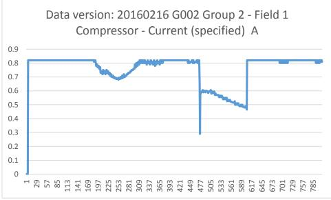
These charts show the delay between request for cooling and the delay. In this case, around two minutes. Gets into the regulation phase (less current than max) when the evaporator is cooled down.
