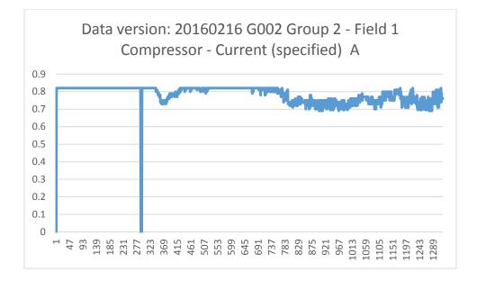
With this scale, it is easier to see the details of compressor current. The drop to 0 is from my manipulation of the controls
