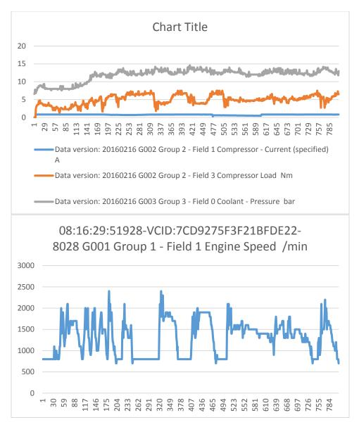
Wanted to show the rpm with the current, pressure, and compressor load. My first impression for the compressor load is it scales with the pressure, but is reduced at higher rpm.
