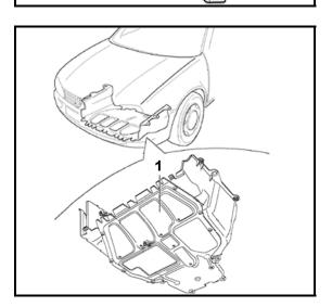
Raise vehicle and remove engine sound dampening pan -1-
