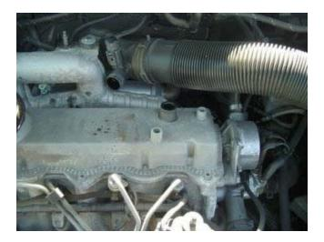
Notice the two locating raised plugs on the cover. There is a plastic plug on the bottom of the CCV that fits into one to keep it located. It will have started in the one on the left front, when we re-install the CCV we will locate it in the one on the right back. It is very easy to see also in the first picture.
