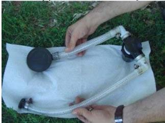
Simply re-install the CCV into its location, remembering to locate the pin in the right hand side hole instead of the original left, like this (shown with EGR fitting still unplugged):
