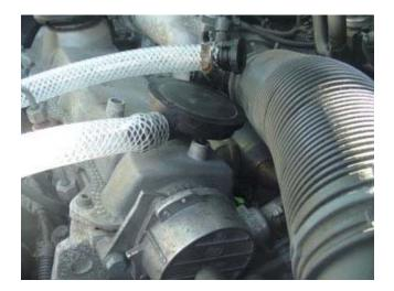
And then plug the EGR fitting back onto the EGR.
