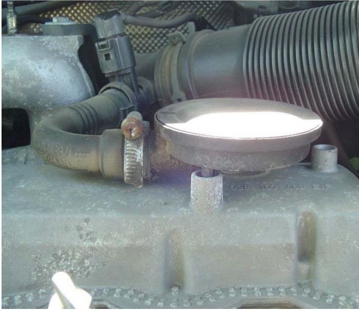
Loosen the clamp that clamps the plastic tube to the CCV, and remove the plastic tube from the EGR by squeezing the two tabs and pulling off.
