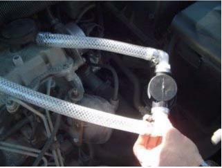
Position the KCTDI-CCV out of the way of the cover bolt. At this point, you have the option of either leaving it under where the cover will go by keeping it to the left of where it is in the picture and left of the bolt, or out to the side once the cover is re-installed by locating it as in the picture.
