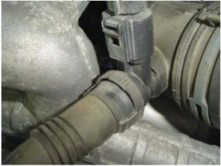
Next, pull the plastic end out of the tube (for clarity we will call it the EGR fitting) - it may already have come off when you removed this tube anyway. Remove the rest of the tube now from the CCV. Keep the end you just removed, along with the clamp that was on the CCV end of the tube, and store the plastic tube with the rest of your "spare parts". Pull the CCV out at this point, it just pulls straight up.
