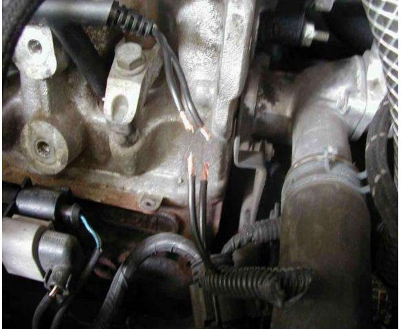
Then crimp on some butt connectors to one set of wires. I use uninsulated ones since I can get a better crimp with them. They will also look nicer (less bulky) under the heat shrink tubing. I got them from Radio Shack:
