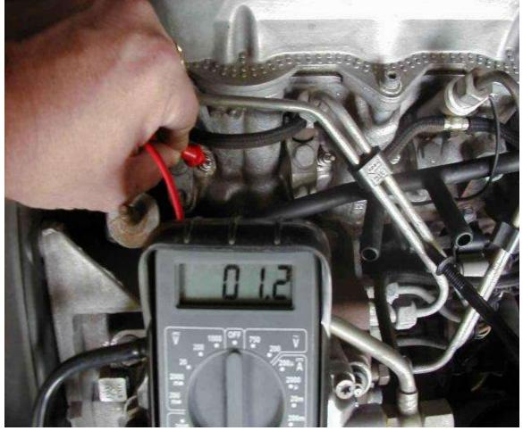
Do this for each plug and take note of the resistance value of each plug. They should all be between 0.5 and 1.5 ohms. It doesn't matter what the readings are, as long as they are close to eachother (within 0.2 - 0.3 ohms). If you have a plug that reads high or infinate, then you have found the bad plug and it needs to be replaced.
