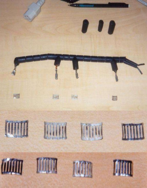
As you can see, the oxidation on the two center liners was quite evident. They are white in color instead of shiny like the outer ones. The poor contact created by the oxidation caused arcing when the voltage was trying to complete the circuit. The
