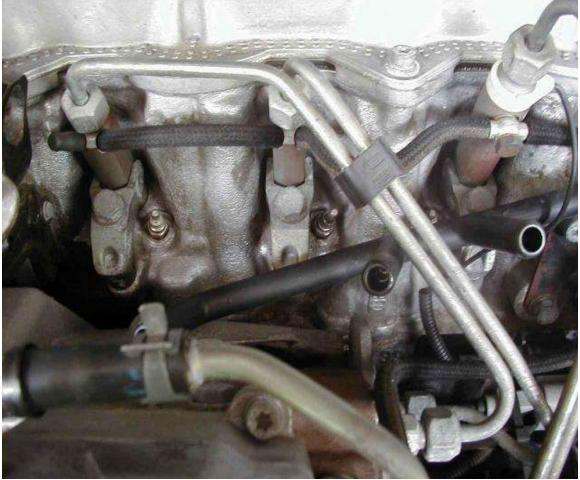
Then get your digital multimeter (available at any auto parts store or Wal-mart for less than \$20) and set it to the lowest ohm setting possible (usually 200). Then place one probe to a good, clean ground and the other probe to the tip of the glow plug:
