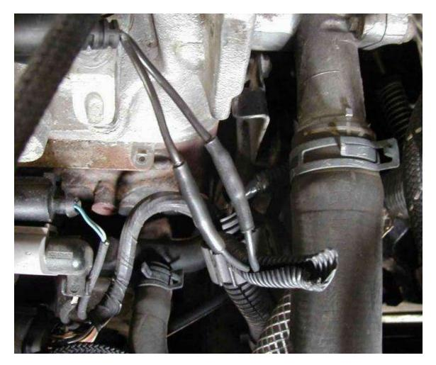
I used heat shring tubing with a glue lining. When it shrinks, the heat melts the glue and it makes a water tight seal around the joint. I bought it at a tractor trailer repair shop. They use it for wiring trailers since the wires are exposed to the elemnts (rain, snow & salt). They are very good. You will also find it easier to do the crimping if you remove the vacuum ball and set it off to the side. There is more room to get the crimping pliers in there.
