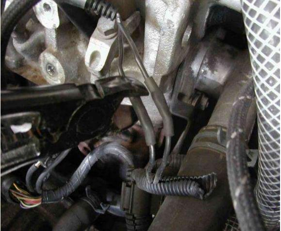
The new harness (two wire version) comes with spade connectors on the endes of the leads. Just cut them off since there is nothing to connect them to anyway. Then strip about 1/4 inch off each lead:
