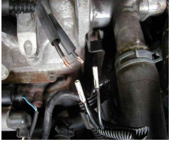
Then I slid on a couple of pieces of heat shrink tubing and crimped the other two wires to complete the splice:
