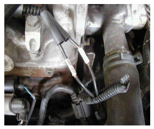
I then used a heat gun to shrink the tubing to seal the joint:
