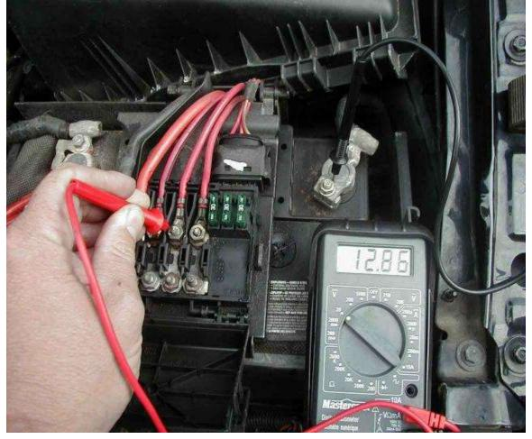
In my case, I got no reading on the far side of 2 of the links. The glow plug fuse is the second from the right. I removed the fuses, cleaned them with sandpaper and reinstalled them. I also used some Deoxit D5 to help enhance the contact & remove the oxidation. If your fuses are clean looking, I wouldn't worry about it, but it can't hurt to check. Of course, if one is blown, then replace it.
