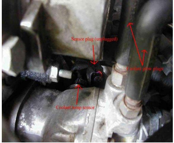
It is located in the housing below and behind the 3 coolant glow plugs(manual transmission cars). It is difficult to see, so you may have to feel for it. It unplugs in a similar way the MAF unplugs, just a smaller plug. You need to push on the tab with your thumb to release the clip while wiggling the plug off . Practice on the MAF if you want to get a hang of it.
