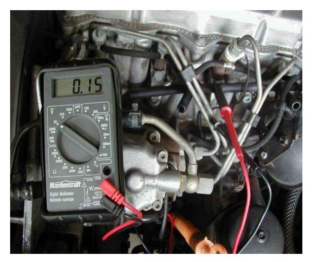
I'm not sure why there is still voltage, but it is normal. If you do not get 12V at any time, then your relay is not completing the circuit and needs to be replaced. The relay is an expensive part (around \$125), but fortunately, it is not often the cause of the code. I have only tested one system out of dozens that I have tested that ended being a relay problem.
