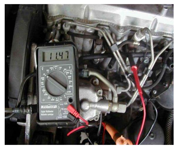
You should get around 12V at each finger of the harness. The glow time is only about 20 seconds, so you may have to repeat the procedure to get all four if your not fast enough. Once the glow time is up, the voltage will drop, but it will still show a small votage at the harness terminals:
