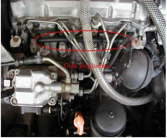
To remove it, just hook your finger under each terminal and pull. they snap on & off like spark plug boots. Once it is off, just rotate it out of the way so you can expose your plugs:
