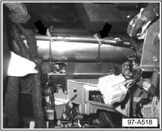
Route antenna along body cross member and attach using two plastic tie straps -arrows- Part No: N 020 902 2 to the two bands around the cross member as shown.
