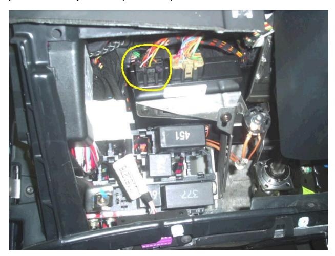
The BLACK connector that is circled above is the the connector that houses the antenna wire. unplug in and pull it down the best you can to get to the wire.
