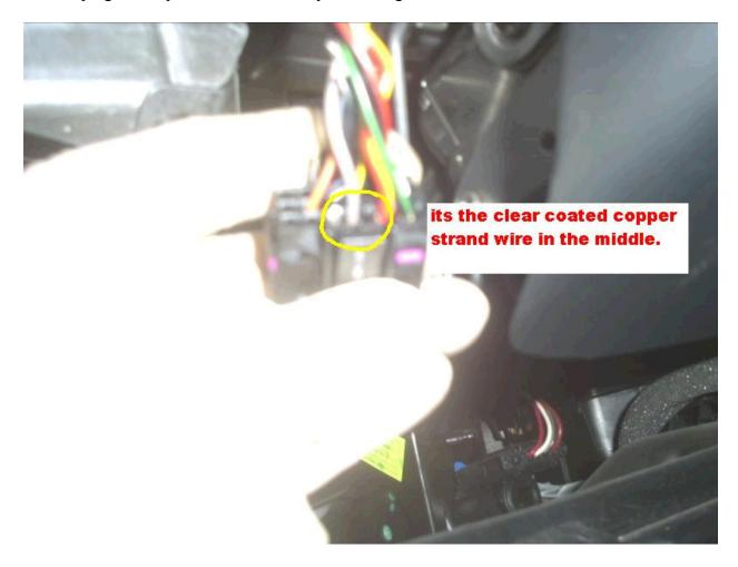
Now you have to push the purple terminal lock to the side in order to remove the old antenna wire terminal. you will need a special wire removal tool. \*(as i said before it will be difficult for some of you to find one, so if you want to skip removing the entire wire and want to TRY and cut the antenna wire and splice new wire to the old terminal still in the connector then go for it!)\*
