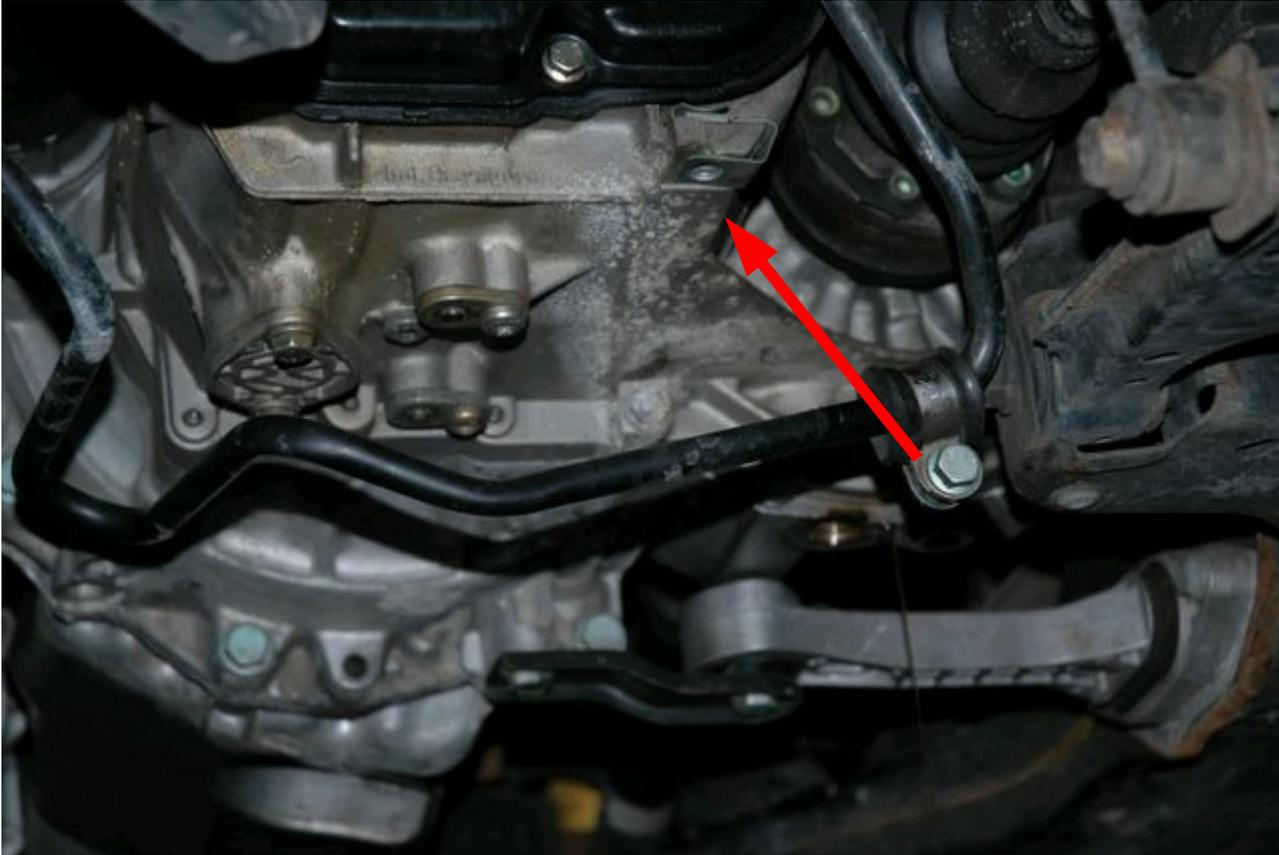
Then looking in from the wheel well you want to remove the bolt that holds the same line to the bottom of the transmission.
