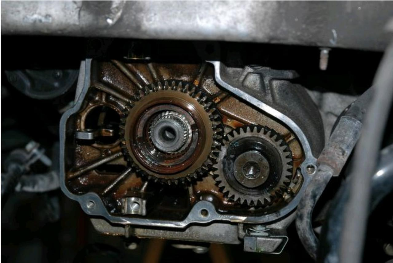
With the big gear off this is what you should see. The syncho and 5<sup>th</sup> gear along with the needle bearing it rides on will just slide right off now.
