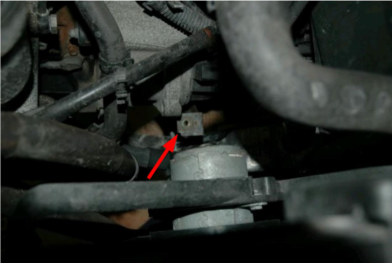
This is looking overhead into the engine bay. You want to remove the bolt that holds the power steering line here. This line kinda gets in the way of accessing the tranny.
