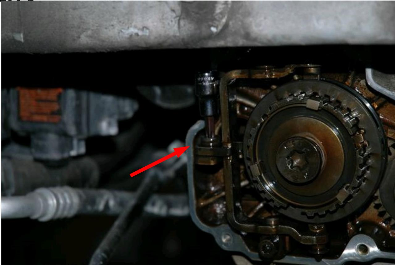
Once the endplate is off you will want to remove the small bolt that connects the selector to the selector shaft.
