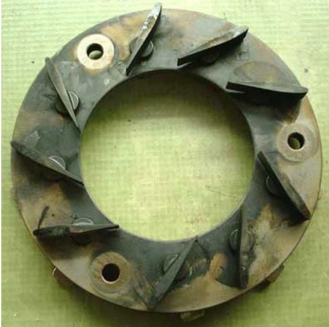
The vane side of the VNT mechanism, showing the narrow vanes and the three holes for the screws. Brass spacers fit over the screws and allow the vane plate to be screwed down without the vanes coming into contact with the machined plate.
