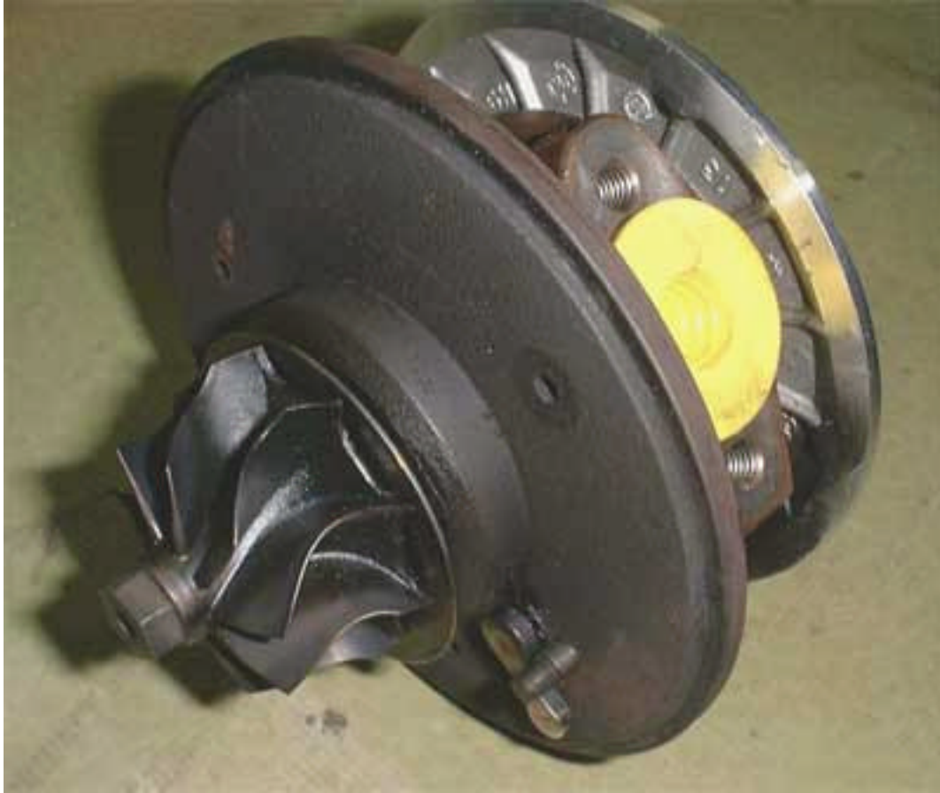
A clean turbo ready for re-assembly. The yellow plug is in the hole for the oil return line.
