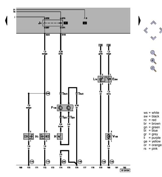
Dual tone horn, tank flap remote unlocking, horn operation
