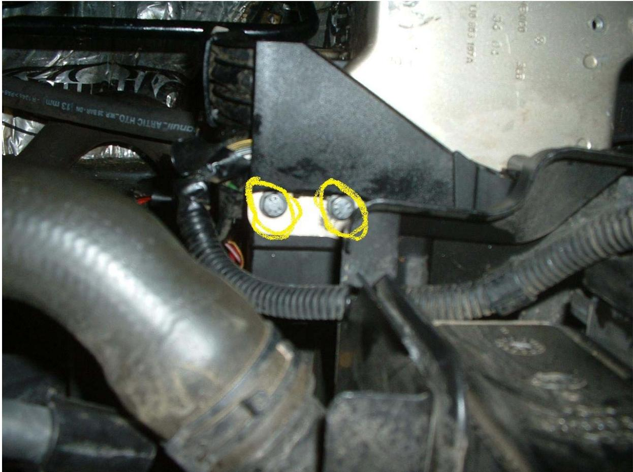
These are the only two bolts that hold the Fan Control Module in place. They are just forward of the battery box. The battery box is removed in this photo (which was taken while cleaning grounds.)
