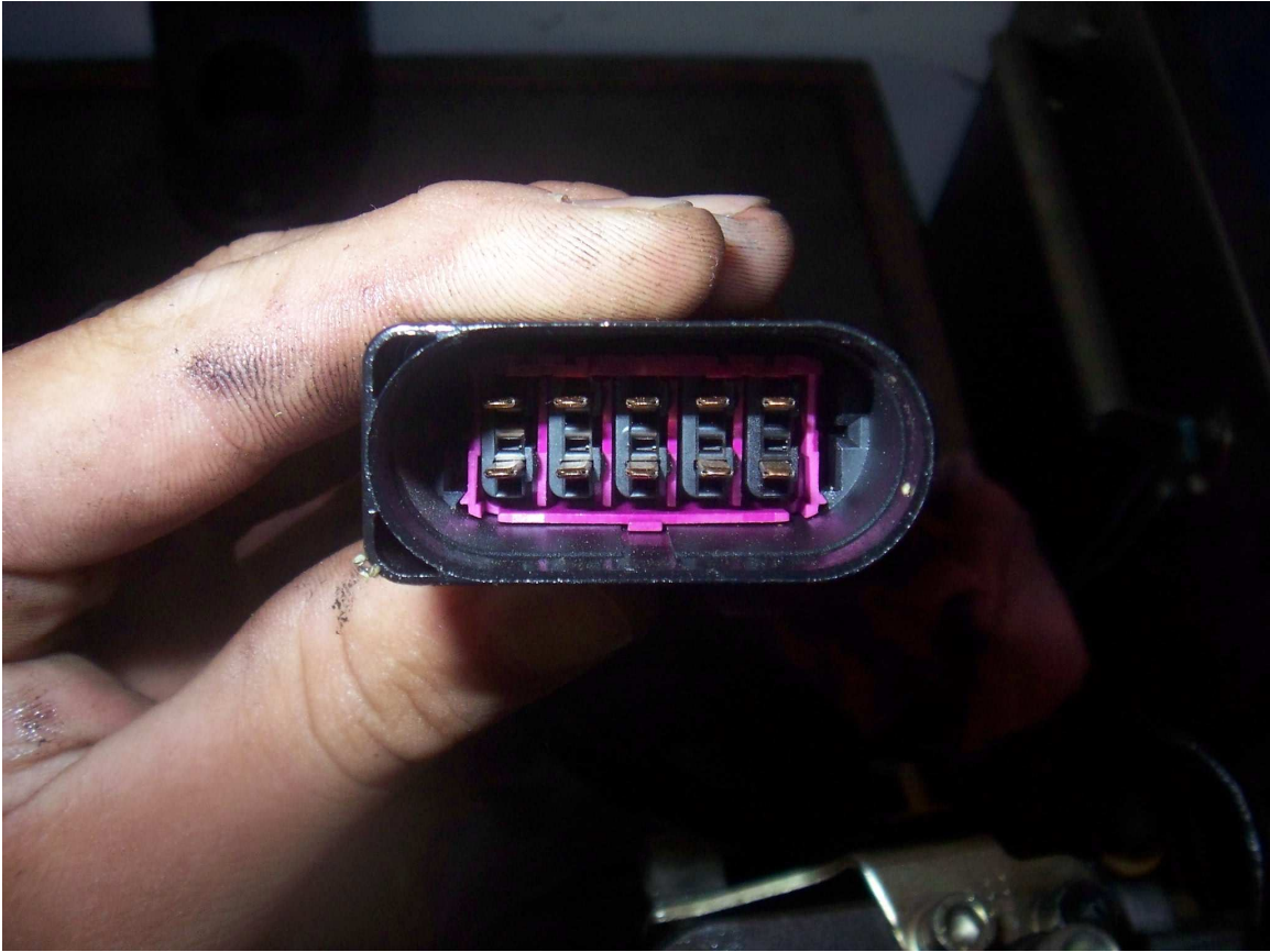
Fig. 5 The open position of the connector lock.
