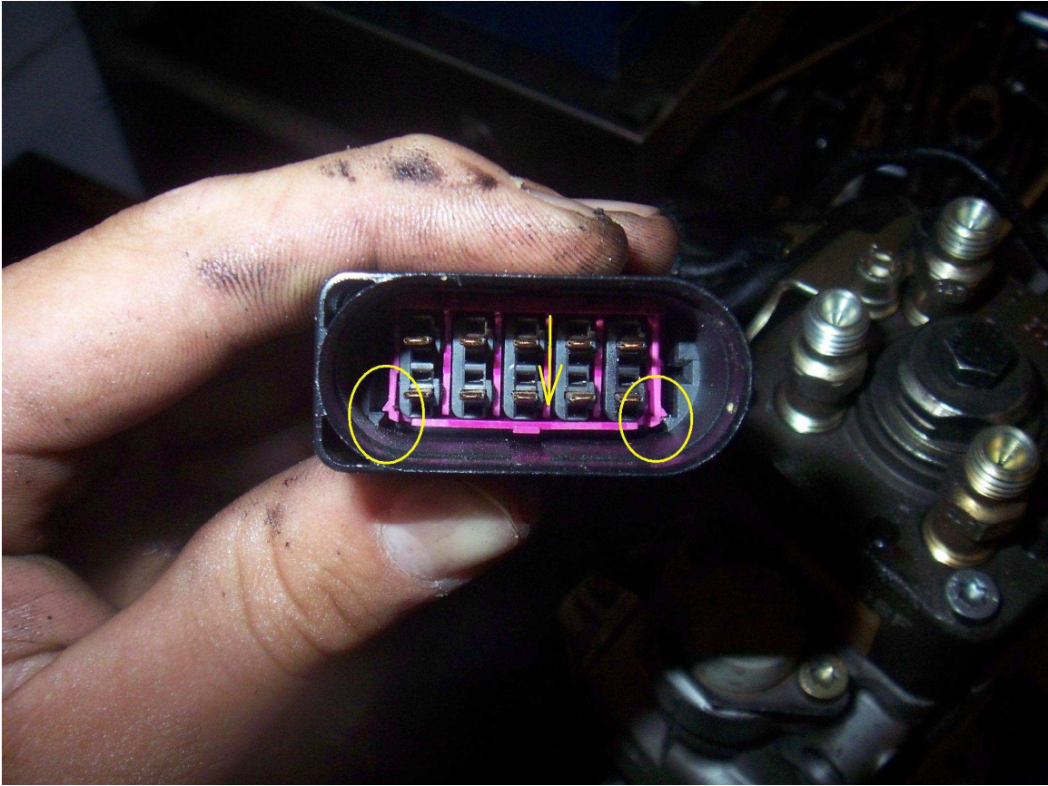
Fig. 4 The installed position of the connector lock.
