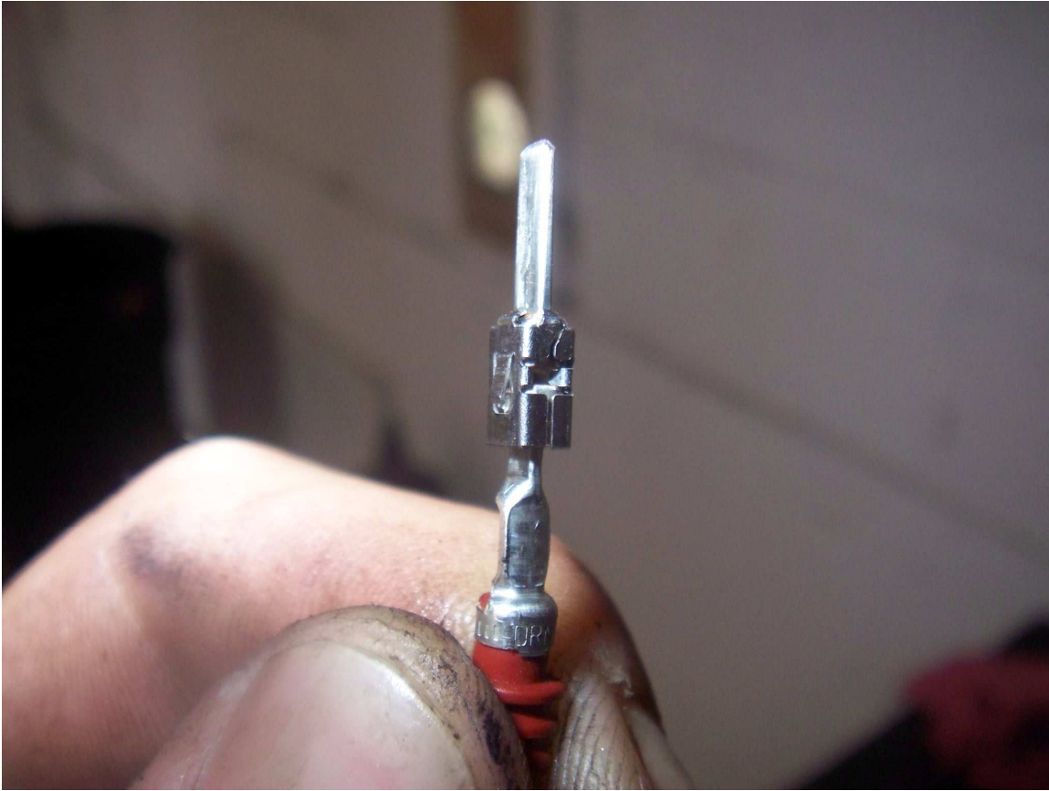
Fig. 7 A removed spade. The tool depresses the metal tabs on the sides of the spade to release it from the plastic connector.
