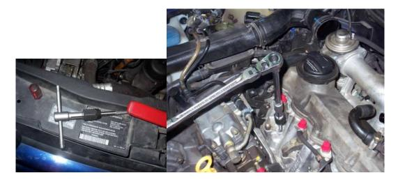
Install a new glow plug. Use anti-seize, and torque to 11ft-lbs.
