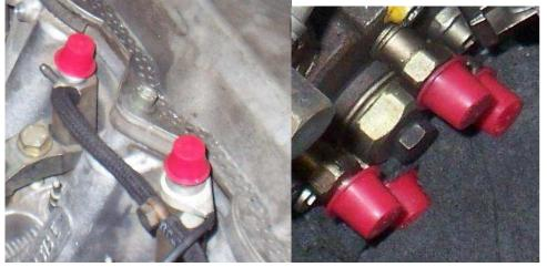
Remove the injector retainer nearest the siezed plug using the 13mm socket, extension, and ratchet.
