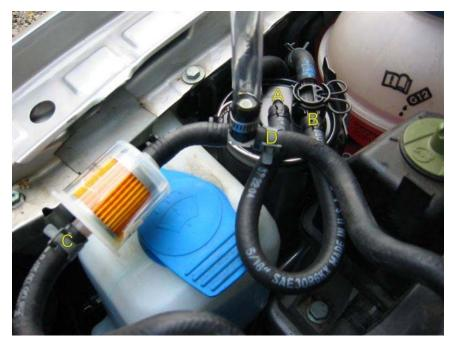
1. Remove the Fuel Return Line (D) from fitting B and connect it to the T fitting.
