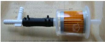
A. Using one of the short sections of fuel hose and two of the hose clamps supplied with the Purolator fuel filter, connect the T with the fuel filter.
