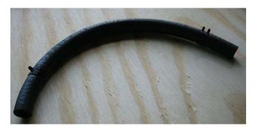
C. Make a Lift Pump Return Line [Only for 04 and Later TDI engines, earlier models were not equipped with lift pumps]
