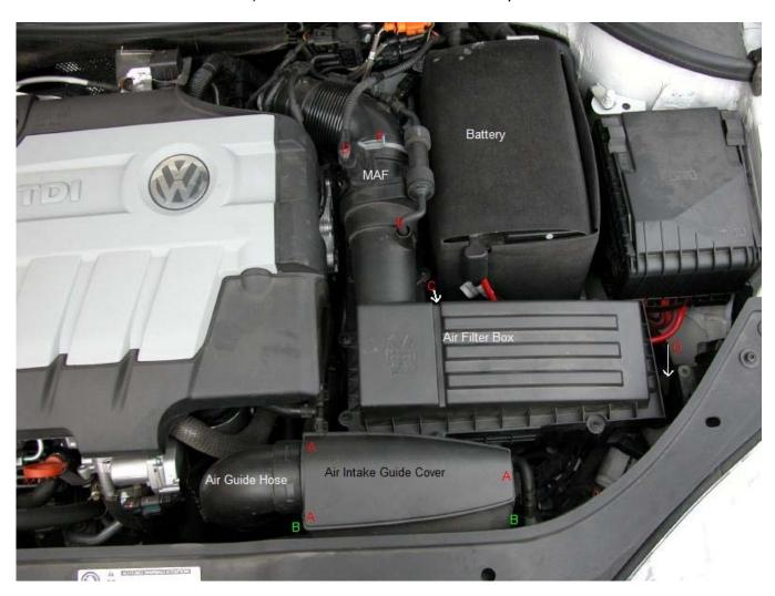
First remove the cover to the "intake air guide" (there are three little plastic clips at locations marked "A" in pic above). This is right at the front of the car right behind the left side of the radiator (see above). Then, there are two plastic clips on the sides of the air guide bottom
