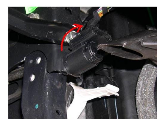
7. Connect the wiring harness to the switch, as shown in the picture below. The switch has been installed correctly and should now work fine.
