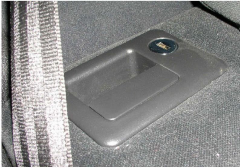
Insert the correct key and rotate the cylinder 90 degrees so that it is halfway between the locked and unlocked positions.
