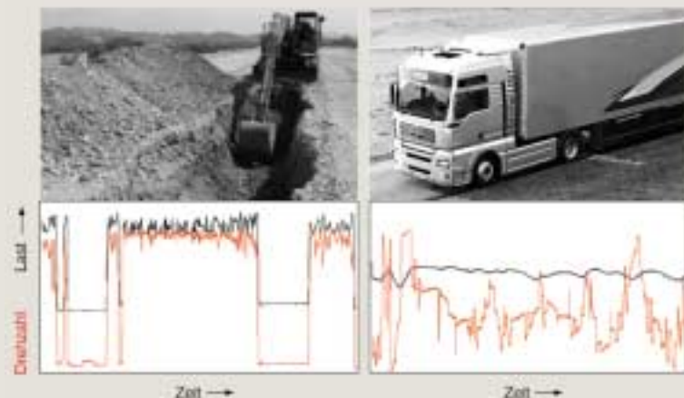
Bild 18: Vergleich von typischen On-highway-/Off-Highway-Lastkollektiven Figure 18: Comparison of typical on-highway/off-highway load maps
