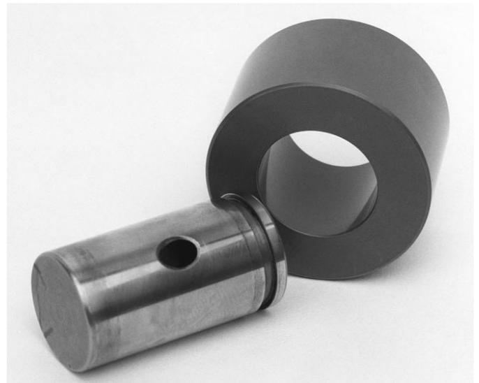
**Figure 51** – Silicon nitride roller and steel pin after 4,000 hours durability testing.
