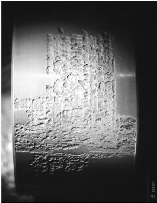
**Figure 57** – Experimental ceramic roller operating at too high an Hertzian stress.
