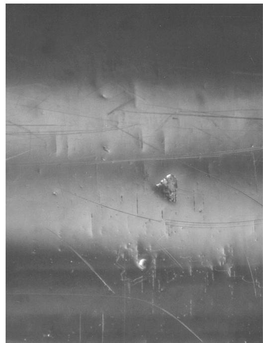
Figure A-3 – Engine cam showing surface glazing in V-8 engine. Surface is fully flooded with oil.
