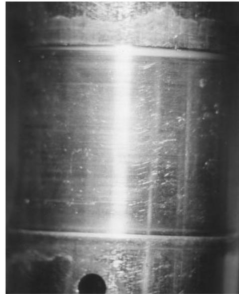
**Figure 45** – Exhaust roller bronze pin showing wearstep.
