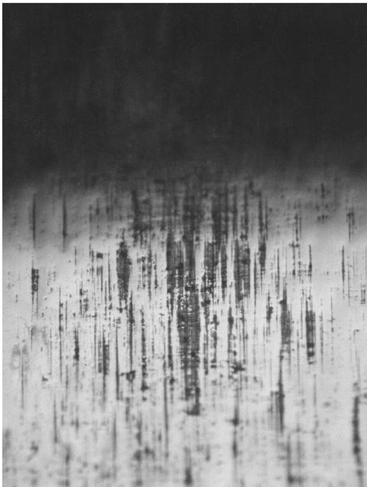
Figure A-2 – Engine cam showing surface glazing in V-8 engine surface fully flooded in oil.
