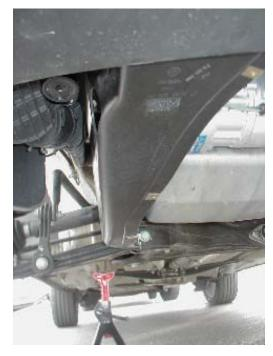
12. Once the side panels are in place. You can see where the mounting arms of the new belly pan go through the new side panel and mount to the bracket.
