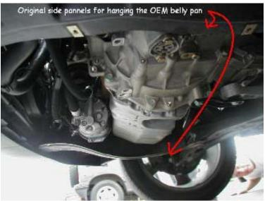
5. We then removed the old belly pan and began removing the old side panels. In the front and rear (outside side) of the side panels, there are press-on connectors on threaded studs. You can either work them off gently or use a small screwdriver to unscrew them. They are a pain in the butt either way.
