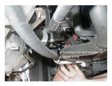
10. Be sure to tighten the post screws well. This secures your belly pan to the car, and you don't want that shaking loose.
