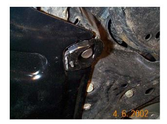
16. Go around and tighten up all the screw/bracket connections. (Thanks again to VWVet for the pic from his install.)
