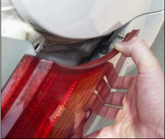
7. Now, rotate the light assembly downwards to gain access to the light assembly itself. The light assembly will snap off of the back of the plastic tail light assembly housing.
