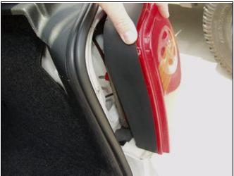
6. Now, we are going to pull the assembly out to the right of the vehicle. This is in a direction 90 degrees to the front of the vehicle. Move the back of the light out about one inch (as done previously). Now – grip the corner of the light as shown below. Pull 90 away from the vehicle – this is to the side. Pull straight – do NOT twist or pry the light. The pin at the corner of the light is pressed into a rubber grommet.
