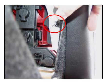
5. Gently press the assembly back towards the rear of the car from the inside. We only need about one inch of clearance. NOTE: You are NOT removing the assembly yet! There is still a pin in the way that we have to deal with (otherwise, you will crack your tail light assembly).
