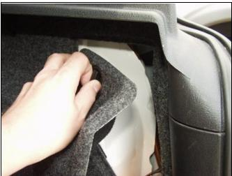
2. Locate the 8mm nuts that we are going to remove. There are 3 on the passenger side. The first is visible right when you take the cover off. Remove it.
