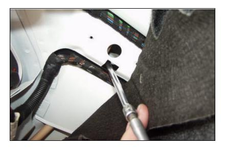
6. Remove the top nut, and the one at the back by the trim (just like the other side). This one is easy because you have pulled back the trim to expose the location.
