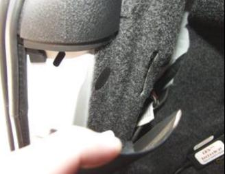
3. Then, we remove the black retainer that holds the carpeting in place where you just pulled the trim back. I am pointing at it with a screw driver for identification only, you must just pull it away from the metal with your fingers. They are just pressed in.
