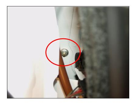
4. The third nut on the passenger side assembly is located just behind the carpeted trim. You have to look back towards the rear of the car to see this one. Remove it.
