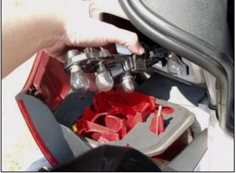
9. Assembly is the reverse of the above steps. NOTE: when reseating the plastic trim, the seal for the rear hatch may get pinched underneath the plastic trim. Just replace it and take a look at the passenger side trim so that the rear hatch gasket is properly seated (this will be obvious when you do it.... Always pay attention to the little details).
