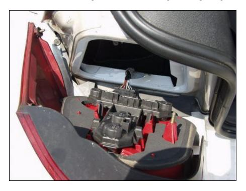
8. Remove the lighting assembly from the housing. Replace the housing with the new housing. Again, I would recommend using a new gasket in the new assembly. This is also a good time to replace bulbs too!
