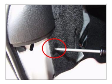
4. Now, pull the carpeting back to gain access to the lower nut on the tail light assembly.
