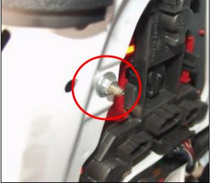
7. Now, we pull the light assembly down and away from the body of the car. There is no pin to worry about on this side, there are 3 bolts and no pin, versus 3 bolts and a pin on the passenger side.
