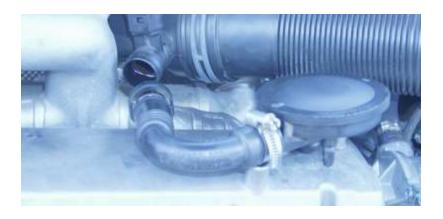
2. Once the hose from the oil/air separator is loose, pull the oil/air separator off the valve cover (this is the round hockey puck looking thing). Remove the grommet. Install the new grommet (help #42052).
