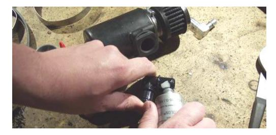
7. Here is the finished product – the elbow should rotate freely with only a medium amount of resistance. The grommet will keep it from leaking, and you can move the elbow around as you need.
