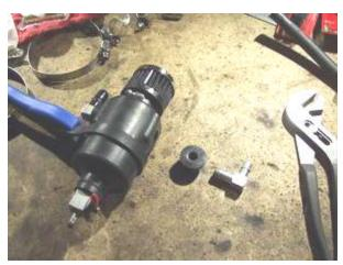
3. We will now use the 7/8" hole saw to cut a hole for the new grommet. NOTE: 7/8" is too small, but it's all I had – so I used a half round file to enlarge the hole just a bit for the grommet to fit. A 1" hole saw would be perfect.
