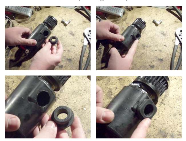
6. Now, put a little grease on the elbow to keep it from binding when you install it, and then just press it in until it seats.
