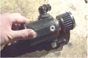
8. Check your work. Remove the top filter; open the drain valve at the bottom and sight down the length of the catch can. Check for obstructions out the bottom valve. You should be able to see straight through if you hold it up to the light. Any debris from drilling might make it drain slow, or not at all.
