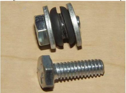
3. BEFORE DRILLING – hold the catch can up against the air box to make sure it is not in the way of anything. Once you find where you want to put it, drill the holes, 3/8" and then install the grommets. Check both sides to make sure the grommets are seated, not pinched, etc. It will look like this when done. Use the bracket that comes with the catch can as a template for how far apart the holes should be.
