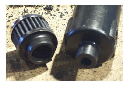
2. I wanted to use some kind of tubing – here is a piece of ¾" PVC in the filter – see how much larger an inner diameter it has. Make sure you check the sizing of the PVC – I was only able to get it in 8' sections – but it's only \$1.50 for that length.
