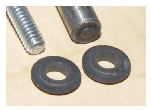
2. Now, you will need a slightly longer bolt. Here is the bolt that comes with the catch can, and two washers and the grommet. Note the longer bolt below it. This is a coarse SAE size bolt. Very common. Not sure what size, because I have a drawer full of them in the garage. You can get them at most hardware stores. Take one of your bolts with you to size the inner diameter of the grommet. If unsure, ask for assistance at Lowe's or Home Depot
