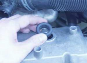
3. OK – here is where we use the modification that Denis at Fred's TDICLUB suggested. Take a pair of pliers – needle nose will work – and pull the quick disconnect from the hose.
