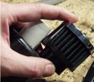
An ALTERNATE method is to get a short piece that sticks just past the grommet on the inside, and just past the neck of the filter. This method should use a VERY tight fit for the PVC into the grommet so the tube does not fall into the catch can. A worm drive clamp can also keep that from happening, or just tightening the clamp on the filter down so that the piece of pipe comes out with the filter.
