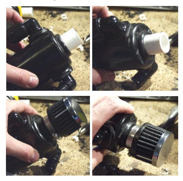
11. The finished top filter modification. Looks like the catch can should have come this way. Larger opening out the top will allow the air to slow down and cool inside the can, hopefully condensing any vapors there instead of inside the filter.
