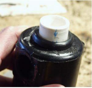
8. Now, we want to get a working piece of PVC. There are several options here for sizing. Using my method, the PVC should bottom out in the can, and stick up through the grommet only enough to fit on the air breather. The picture below is the tube WITHOUT the grommet, which adds about 1/4" installed height to the filter. NOTE: this method is going to require drilling lots of holes in the PVC pipe.
