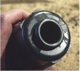
7. Then, insert a short piece of the PVC pipe to check for fitment. You may have to make several adjustments with the file to enlarge the hole. The PVC should fit snugly (when the PVC is not in place, the grommet may appear loose).
