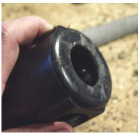
6. Insert the grommet in the top of the catch can in the hole you just made.
