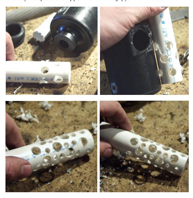
10. Now, we seat the grommet and seat the new modified tube into the catch can. Use of a little grease / oil will keep the PVC tube from binding. It should seat with enough space at the top to install the air filter. (NOTE: I have modified both sides of the catch can for <sup>3</sup>/<sub>4</sub>" hose in case I want to move it later and need to plumb the other side).
