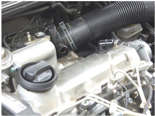
3. Now, attach the hose to the elbow with a worm drive clamp.
