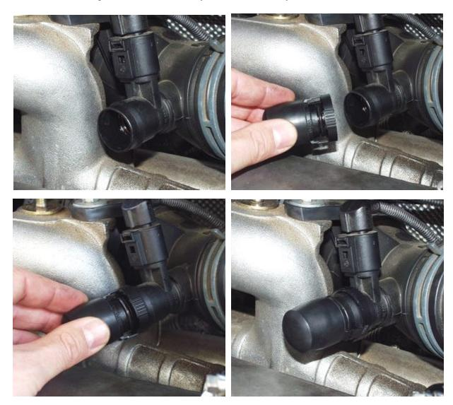
4. Here is a close-up of the capped hole in the intake and the elbow with the hose attached.
