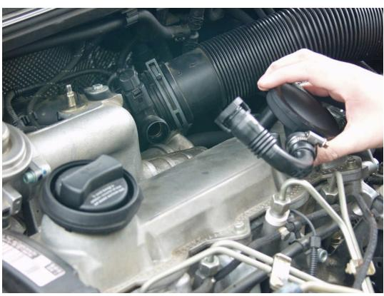
3. Next, we remove the original grommet that is in the valve cover.
