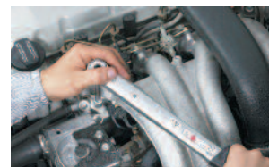
Always use a torque wrench when disassembling and assembling glow plugs.
