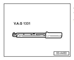
• Install oil drain plug and hand-tighten first. Then, using a torque wrench, tighten to the proper specification as listed in the table below. See \_ <u>Required Parts and Tools</u>.
