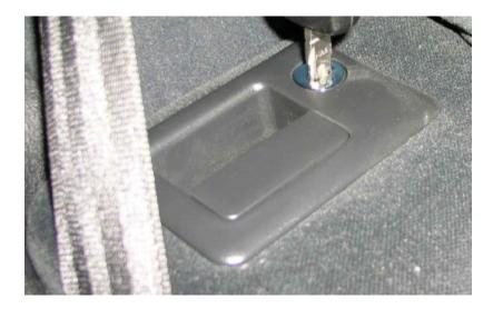
CAREFULLY pull straight up on the key and the lock cylinder will come out of the handle trim plate.
