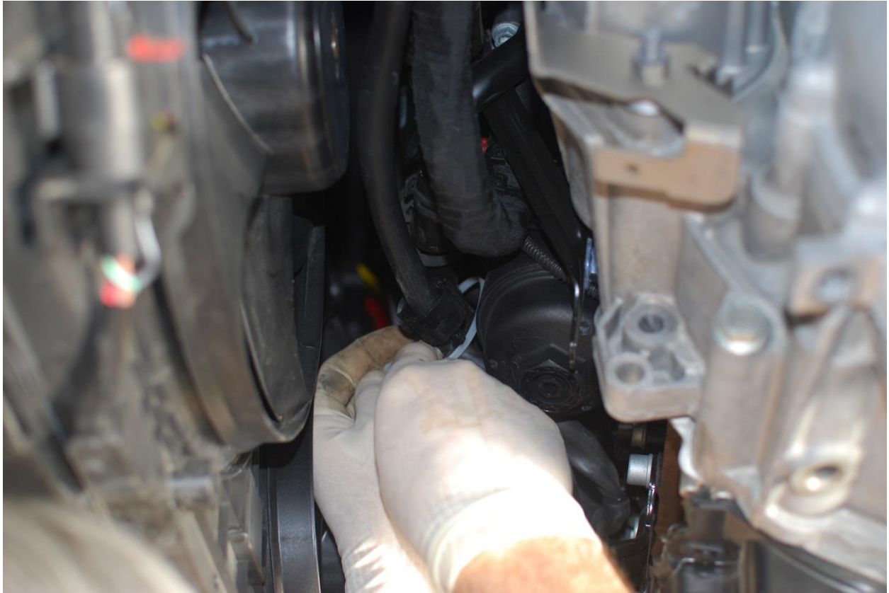
A cable tie placed around a coolant hose keeps the wiring harness out of the way.
