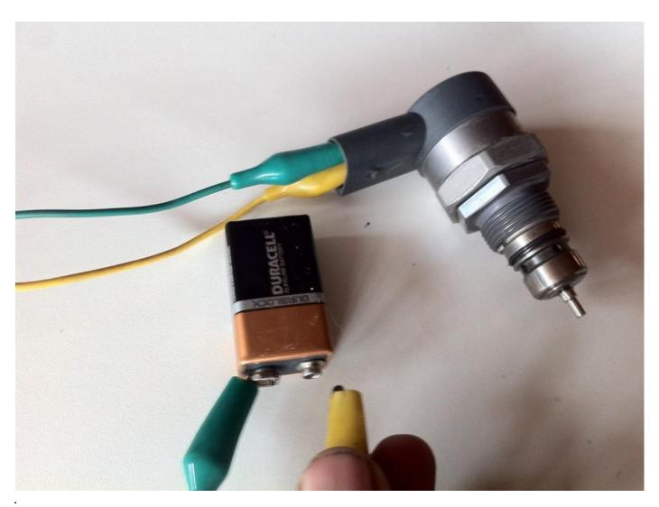
Now with a rubber hose, blow in the end to hear it open and close. Blow air in, while cycling the leads. It will be obvious when it's open and closed.
