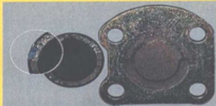
Timing device piston damaged: The use of Biodiesel causes filter plugged, and air comes into VE pump (timing device piston area). It causes the failures.
